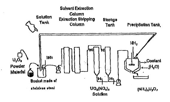
Figure 4. The procedure that was used at the time of the estimating accident. Batches containing 2.4 kgU3Os were dissolved in a stainless steel bucket. The batch was then transferred to a 5-liter beaker and then physically transported to the precipitation tank where it was poured through a function the tank. Seven batches of solution were added to the tank before it went critical.
