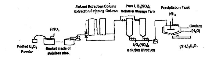
Figure 3. The modified procedure that allowed the use of a stainless steel bucket as a dissolution yessel. The resultant solution was to be pumped into the system for storage in the geometrically favorable solution storage tanks.
