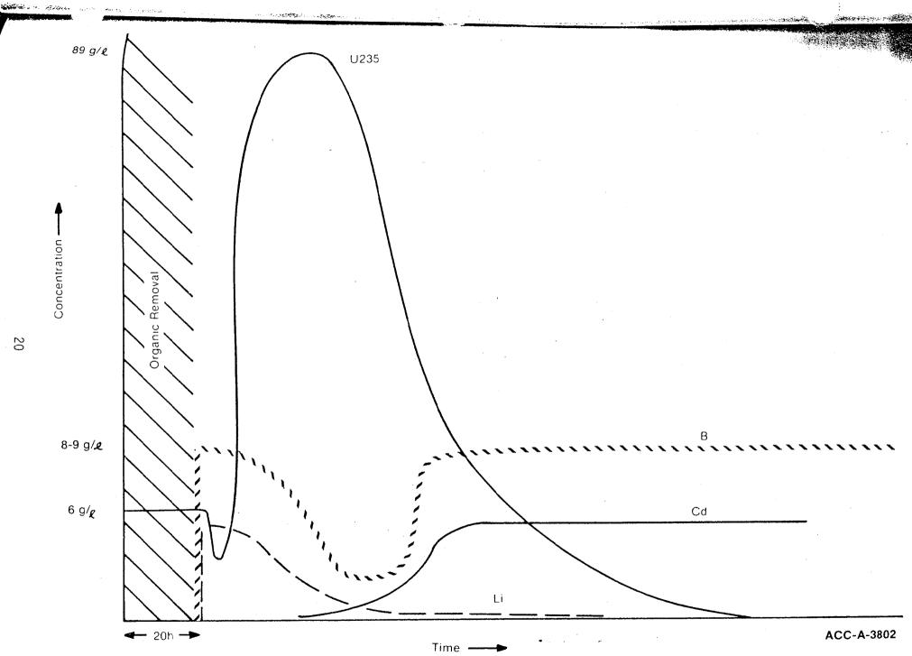
Figure 7. Qualitative Model of Solution Composition During Recovery of Uranium From H-100
