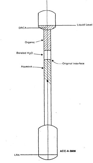
Figure 17 Relation of Borated Water, Organic, and Aqueous After First Borated Water Addition to Top
