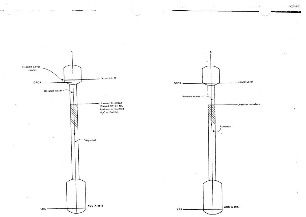
Figure 25 Relation of Borated Water, Uranium Interface, and Aqueous After First Borated Water Addition to the Bottom
