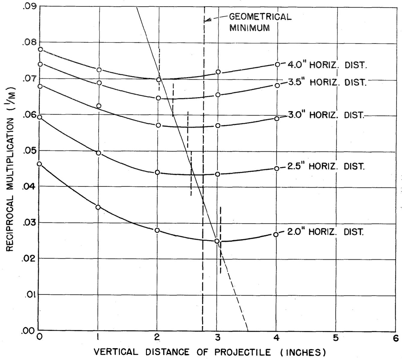
FIG. 5. Plot of reciprocal multiplication vs vertical position of A for various horizontal separation distances between A and B, in effectively infinite water tamping.
