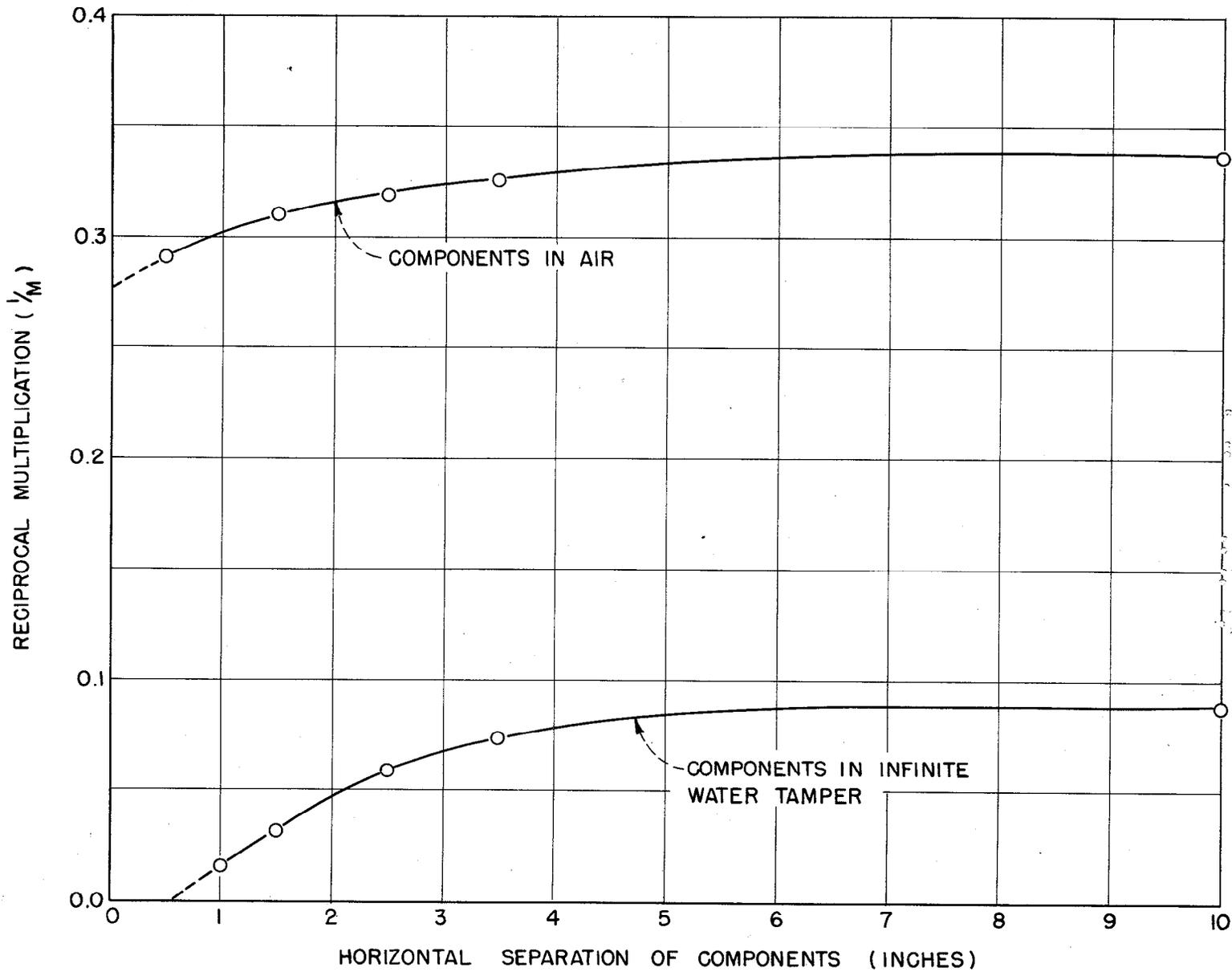
FIG. 3. Proximity measurements on A and B, in air and in effectively infinite water tamping.
