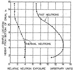
Fig. 8. Relative neutron exposure of samples from side of stainless steel drum.
