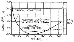
Fig. 2. Mass-volume relations in 55 gal drum during radiation excursion.
