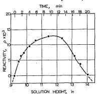
Fig. 3. Calculated reactivity in drum during radiation excursion.
