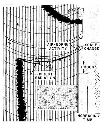
Fig. 6. Recorder chart from air sampler located down wind from accident.
