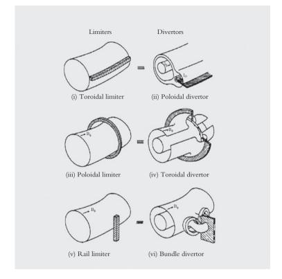
**Figure 2.3** Limiter and divertor configurations. (Note that the circular surface represents the plasma surface for the limiter configurations, and the wall if further outside but not shown. For the divertor configurations, both the plasma surface and outside of it the wall are shown.)
