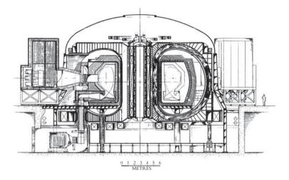
Figure 3.4 INTOR conceptual design (1981). See text for details.
