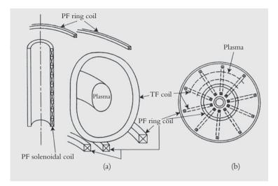
**Figure 3.1** Magnet system configuration of the type adopted for INTOR: (a) vertical cross section showing only a few PF coils, and(b) top view showing only 2 PF coils (b). PF, poloidal field; TF, toroidal field.
