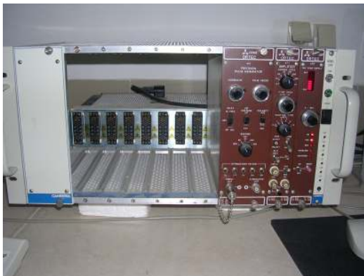
a) Typical NIM-based electronic setup
