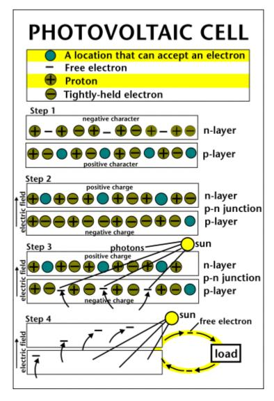
When the electrons leave their position, holes are formed. When many electrons, each carrying a negative charge, travel toward the front surface of the cell, the resulting imbalance of charge between the cell's front and back surfaces creates a voltage potential like the negative and positive terminals of a battery. When the two surfaces are connected through an external load, electricity flows.
