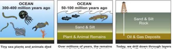
Tiny sea plants and animals died and were buried on the ocean floor. Over time, they were covered by layers of silt and sand. Over millions of years, the remains were buried deeper and deeper. The enormous heat and pressure turned them into oil and gas. Today, we drill down through layers of sand, silt, and rock to reach the rock formations that contain oil and gas deposits.
