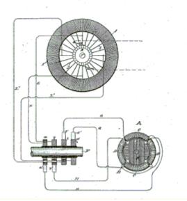
an AC induction motor that produces mechanical energy. Induction motors run household appliances like clothes washers and dryers. Development of these devices led to widespread industrial and manufacturing uses for electricity.
