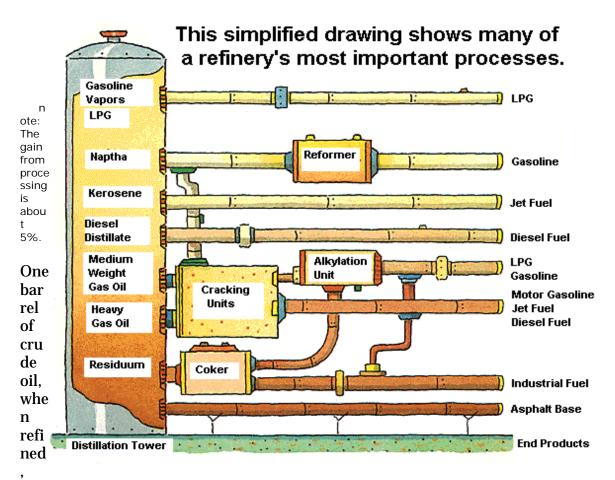
produces about 20 gallons of finished motor gasoline, and 7 gallons of diesel, as well as other petroleum products. Most of the petroleum products are used to produce energy. For instance, many people across the United States use propane to heat their homes and fuel their cars. Other products made from petroleum include: ink, crayons, bubble gum, dishwashing liquids, deodorant, eyeglasses, records, tires, ammonia, and heart valves.
