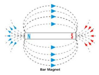
This creates an imbalance in the forces between the ends of a magnet. This creates a **magnetic field** around a magnet. A magnet is labeled with North (N) and South (S) poles. The magnetic force in a magnet flows from the North pole to the South pole.
