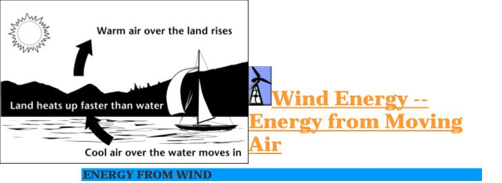
Wind is simple air in motion. It is caused by the uneven heating of the earth's surface by the sun. Since the earth's surface is made of very different types of land and water, it absorbs the sun's heat at different rates.
