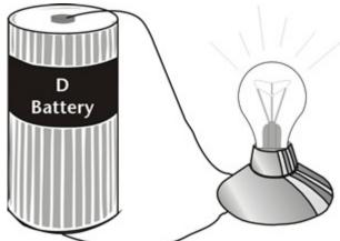
charge. If a wire is attached from one end of the battery to the other, electrons flow through the wire to balance the electrical charge. A load is a device that does work or performs a job. If a load—such as a lightbulb—is placed along the wire, the electricity can do work as it flows through the wire. In the picture above, electrons flow from the negative end of the battery through the wire to the lightbulb. The electricity flows through the wire in the lightbulb and back to the battery.
