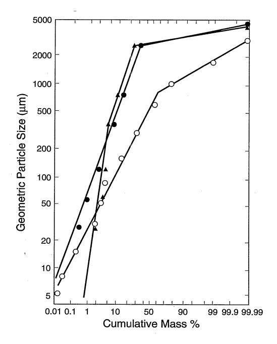
Figure 5. Cumulative mass-size distributions for products formed by corrosion of plutonium metal. Data for products of the Pu+O<sub>2</sub> reaction at temperatures above the 500°C ignition point of the metal [21], the hydride-catalyzed oxidation of Pu by O<sub>2</sub> [4], and the hydride-catalyzed corrosion of Pu by air [4] are indicated by open circles, filled circles, and triangles, respectively.
