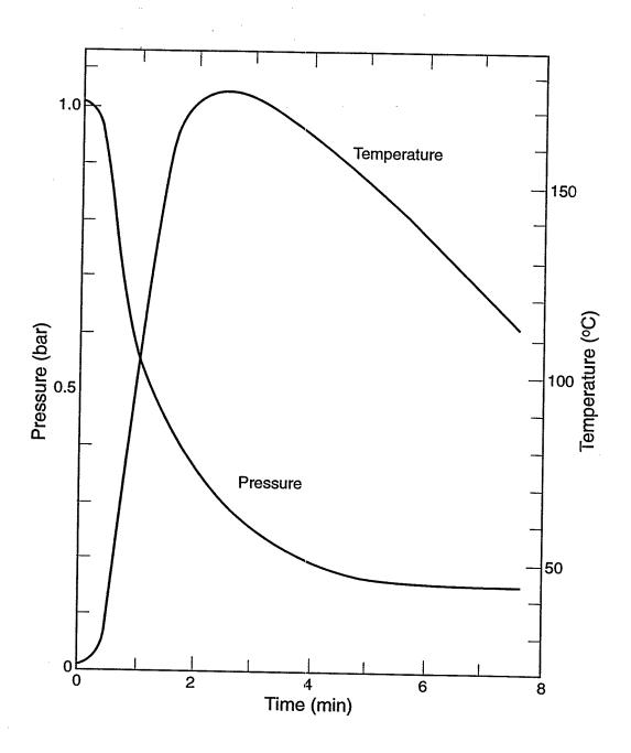
Figure 1. Time dependence of pressure and gas temperature for reaction of air with a mixture of 60% PuOH and 40% Pu in a closed system.
