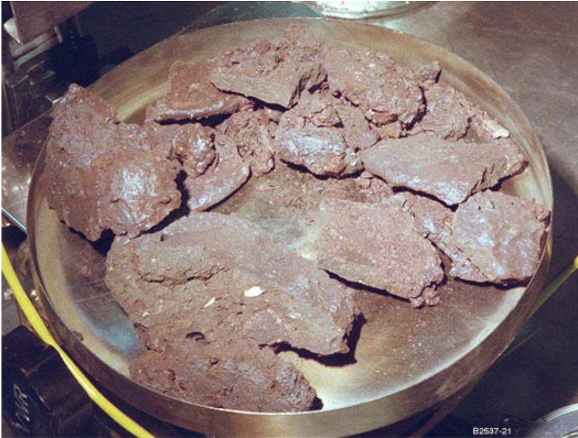
**Fig. 3. ARF-actinide material on the slip top can lid.**
