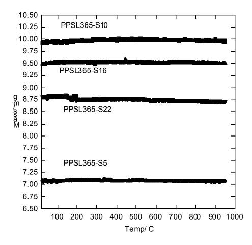
Fig. 4. Thermal gravimetric analysis results for the PPSL-365 samples  $(S_5 \text{ is } S, S_{10} \text{ is } S', S_{16} \text{ is } S'', \text{ and } S_{22} \text{ is } S''')$ .
