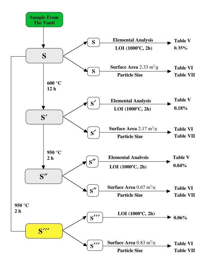
Fig. 2. Characterization of the impure plutonium oxide PPSL-365.
