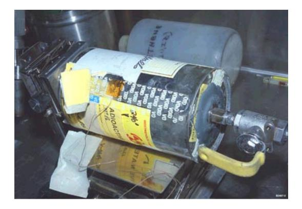
Fig. 1. Puncture device being epoxied to the top of the can.
