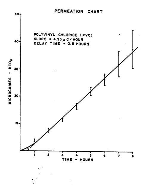
Figure 1 - Hageman Permeation Chart for Polyvinyl Chloride
