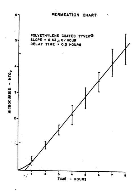
Figure 2 - Hageman Permeation Chart for Polyethylene Coated Tyvek
