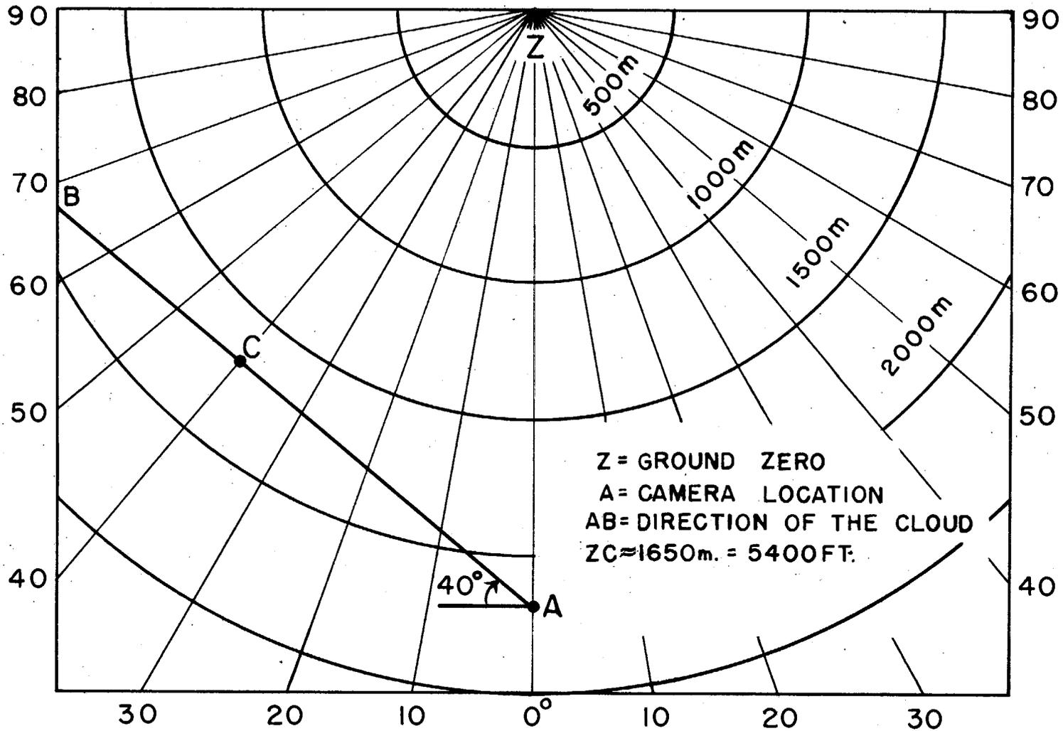
Fig V-1 Position of Camera and Cloud with respect to ground zero.
