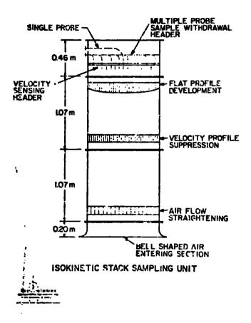
ISOKINETIC SMIPLING PROBE ASSEMBLY
