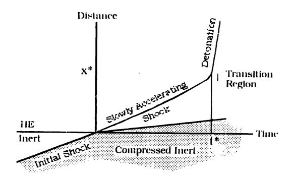
• Induction distance ( $x^*$ ) and time ( $t^*$ ) are a function of Shock Pressure:  $x^*=x^*(P)$ , and  $t^*=t^*(P)$
