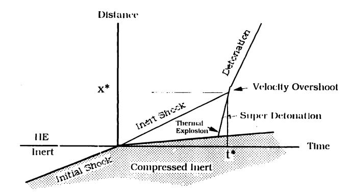
Induction distance (x\*) and time (t\*) are a function of Shock Pressure: x\*= x\*(P), t\* = t\*(P)
