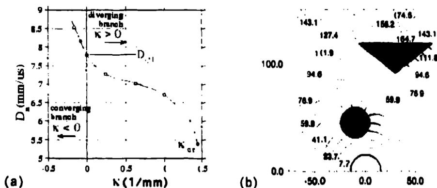
Figure 2. The  $D_n(\kappa)$  for a typical condensed phase explosive, PBX 9502 is shown in Fig. 2a. Burn time contours for an engineering-style problem obtained with the LS-method are shown in Fig 2b. The dark areas are obstacles.
