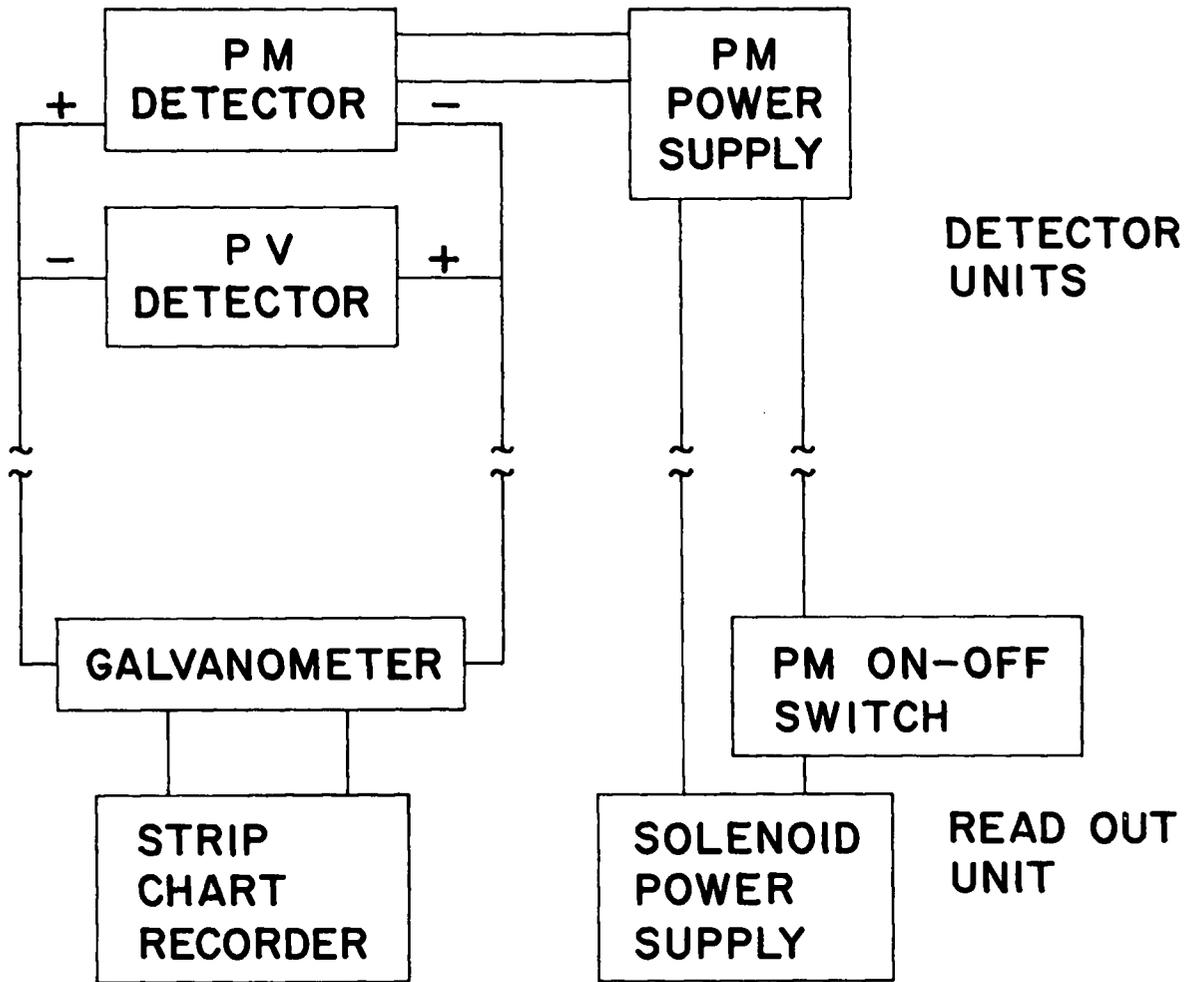
Fig. 6. Block diagram of PV/PM system.
