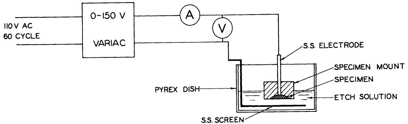
Figure 1. Schematic of equipment used in AC etching. The specimen probe and the mesh screen electrode are made of stainless steel.
