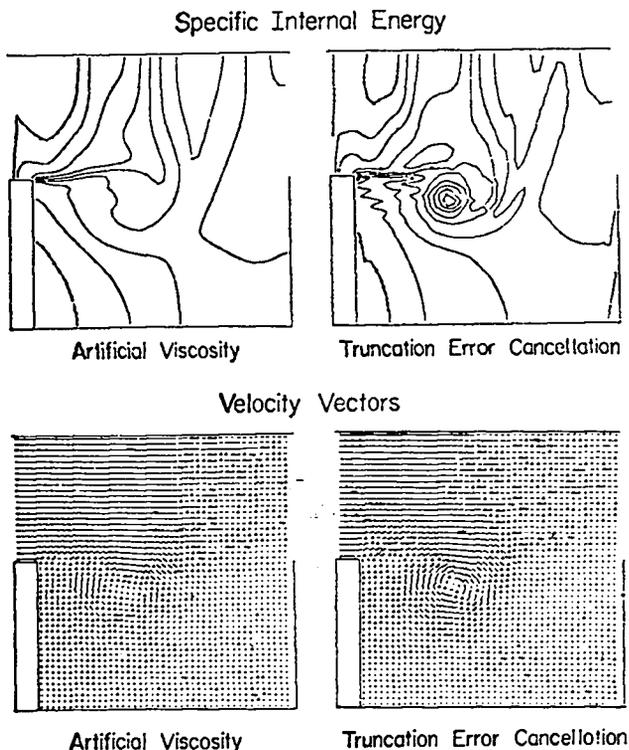
Fig. 4. A two-dimensional flow with and without TEC. The TEC run has 1% as much viscosity as the artificial viscosity run. A Mach 0.1 wind enters the mesh across the upper half of the left boundary, and it leaves across the upper half of the right boundary.
