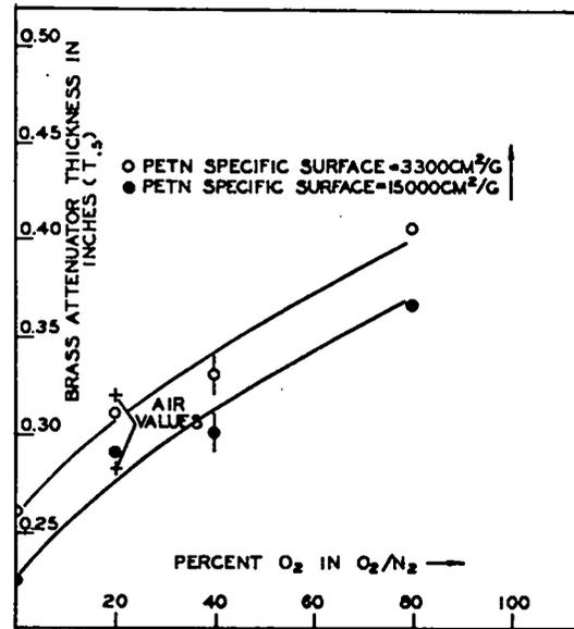
Fig. 7. Effect of oxygen content in O<sub>2</sub>/N<sub>2</sub> gas mixtures on the small-scale gap-test sensitivity of PETN. Total gas pressure = 1000 psig.
