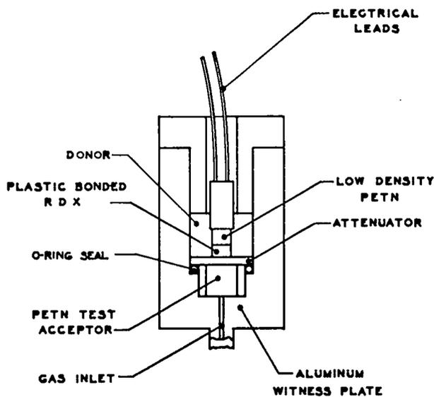
Fig. 1. Assembly for the shock initiation of PETN.
