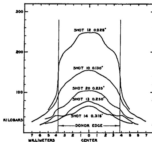
Fig. 2. Attenuator pressure profiles for indicated shots.
