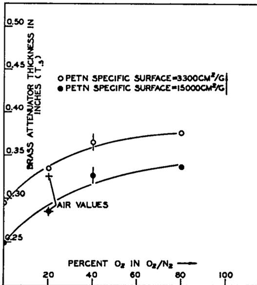
Fig. 6. Effect of oxygen content in O<sub>2</sub>/N<sub>2</sub> gas mixtures on the small-scale gap-test sensitivity of PETN. Total gas pressure = 500 psig.
