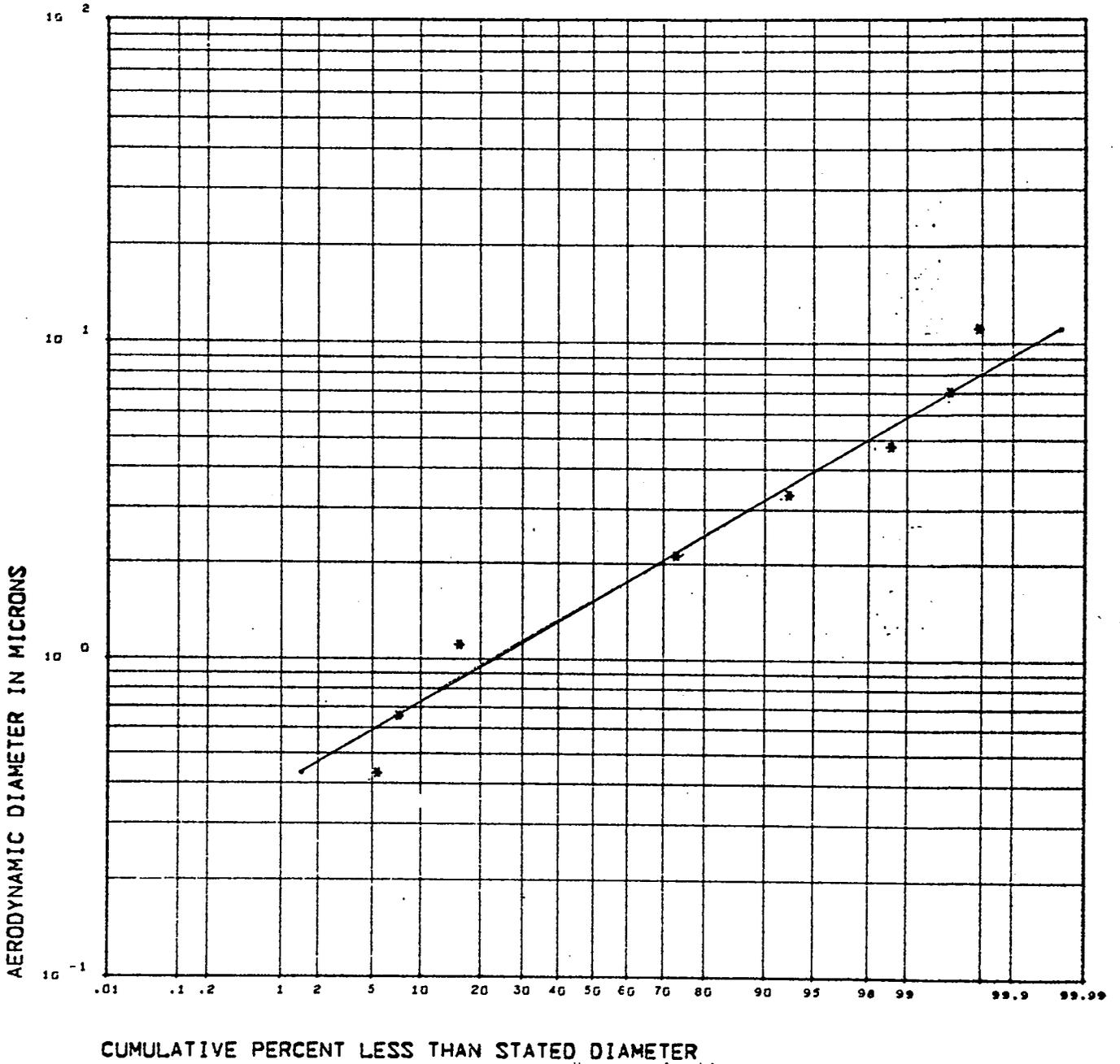
Figure 9: Size Characteristics of Pu Aerosol--
