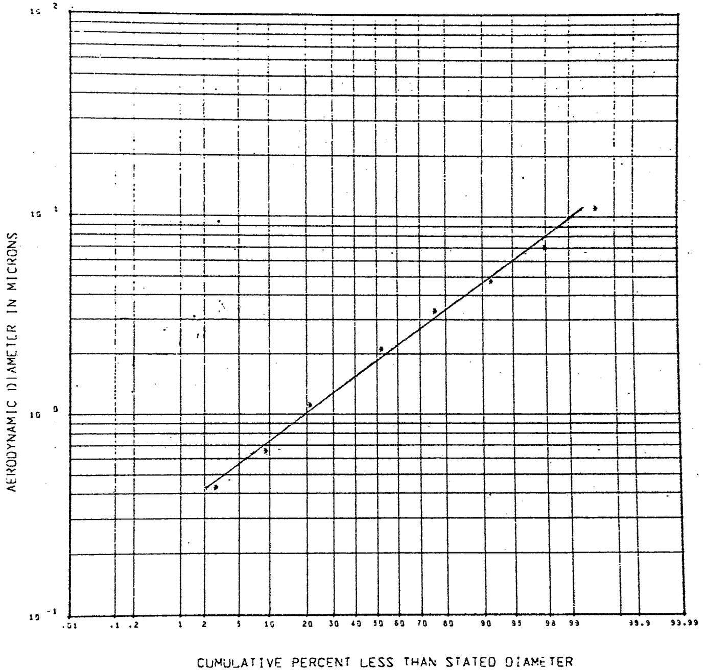
Figure 7: Size Characteristics of Pu Aerosol--
