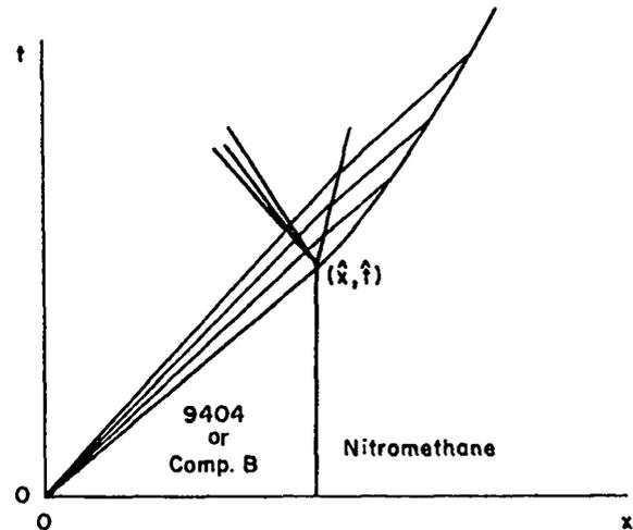
Fig. 1. Overdriven detonation in nitromethane initiated by PBX9404;  $x-t$  diagram.
