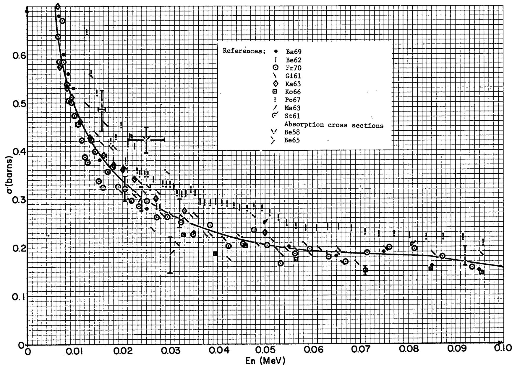
Fig. 1. Natural tungsten smooth radiative capture cross section.
