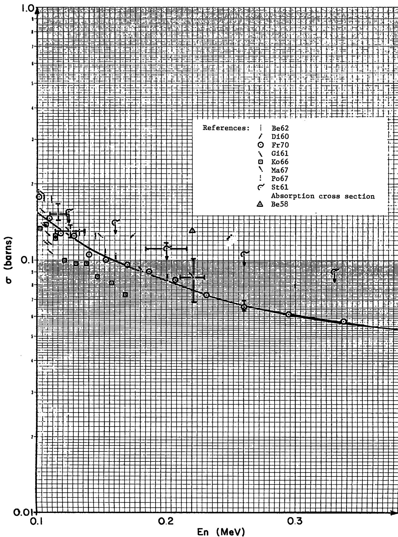
Fig. 6. Natural tungsten smooth radiative capture cross section.
