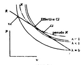
FIGURE 5 Evolution of a pseudo Hugoniot based on an effective CJ state.
