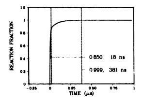
FIGURE 4 PBX 9502 reaction zone showing fast and slow reaction zone thicknesses.
