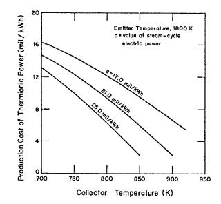
Fig. 13. Production costs of byproduct thermionic power with the value of conventional power as a parameter.
