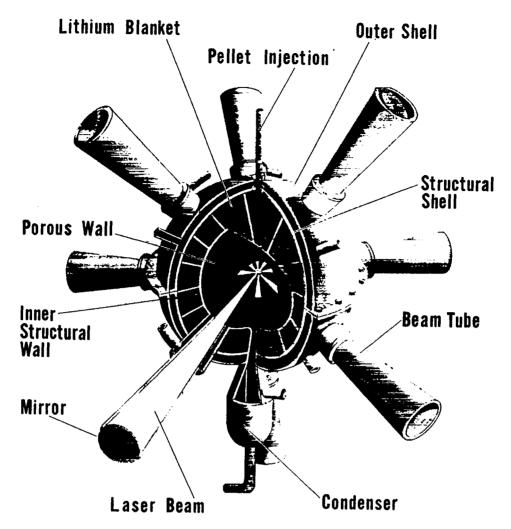
Fig. 1. Wetted-wall laser fusion reactor concept.
