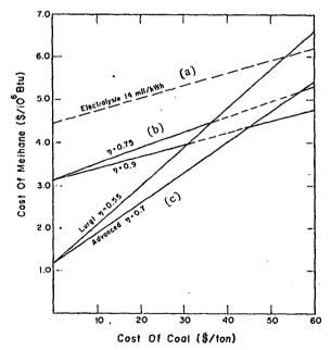
Fig. 11. Costs of producing methane by various methods as functions of the cost of feed coal: (a) electrolytically produced H<sub>2</sub> followed by direct hydrogenation at  $\eta=0.9$ , (b) radiolytimally produced H<sub>2</sub> at  $\eta=0.35$ followed by direct hydrogenation with waste heat converted to electricity and solid for 14 mil/kWh, and (c) standard coal gasification ( $\eta=$ efficiency).
