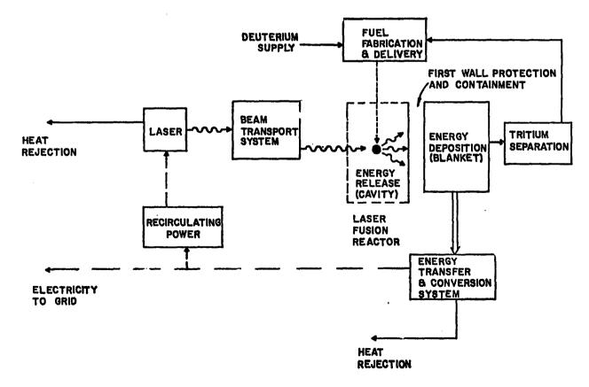
Fig. 3. Schematic energy and mass flow diagram.
