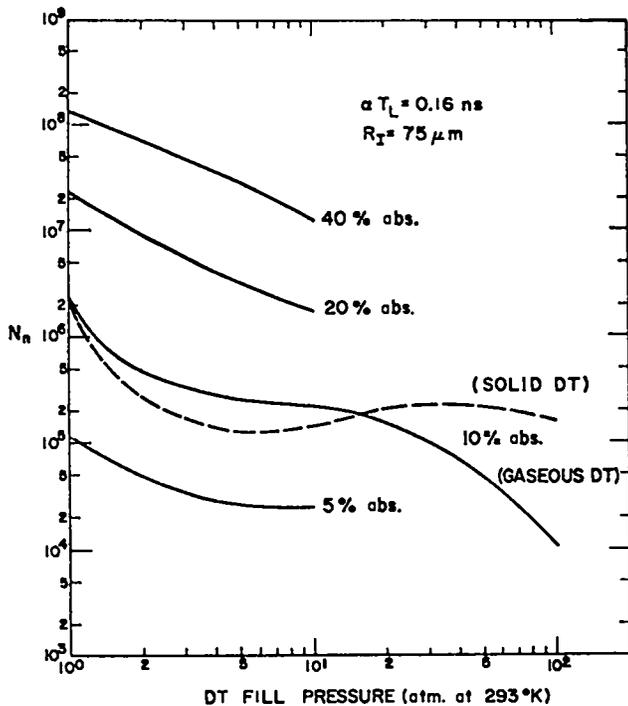
Fig. II.3. Neutrons produced vs. DT fill pressure.
