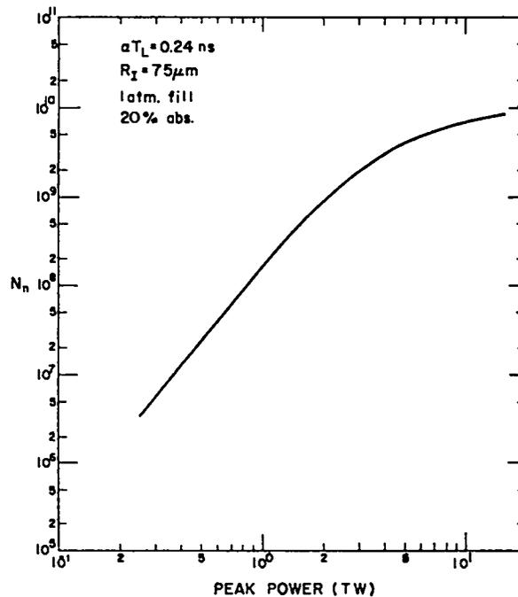
Fig. II.5. Neutrons produced vs. peak laser power.
