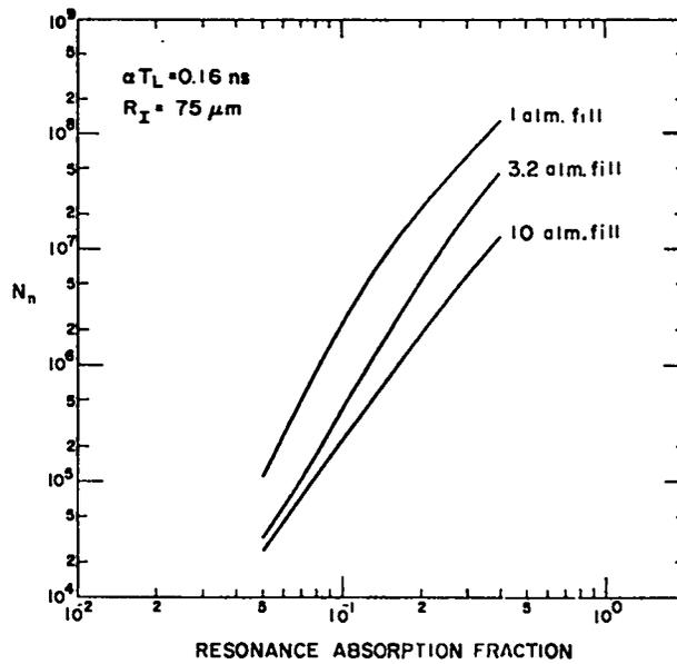
Fig. II.4. Neutrons produced vs. resonance absorption fraction.
