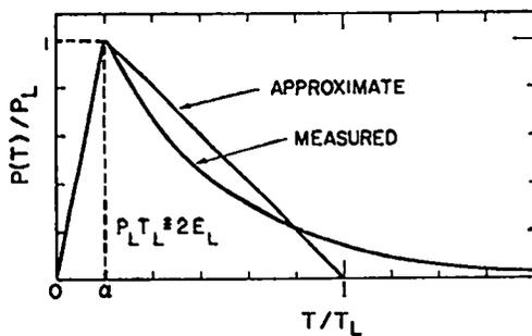
Fig. I.1. Laser temporal pulse shape.
