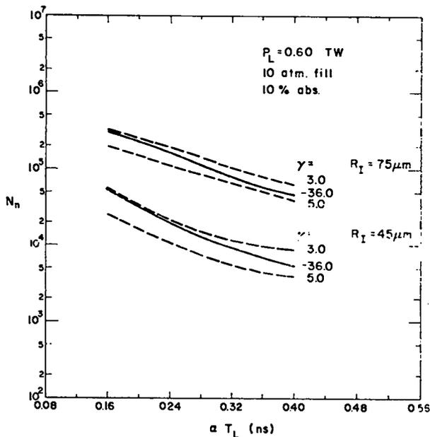
Fig. II.1. Neutrons produced vs. pulse rise time.
