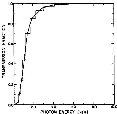
Fig. IV.1. 0.5 mil Be filter transmission function.
