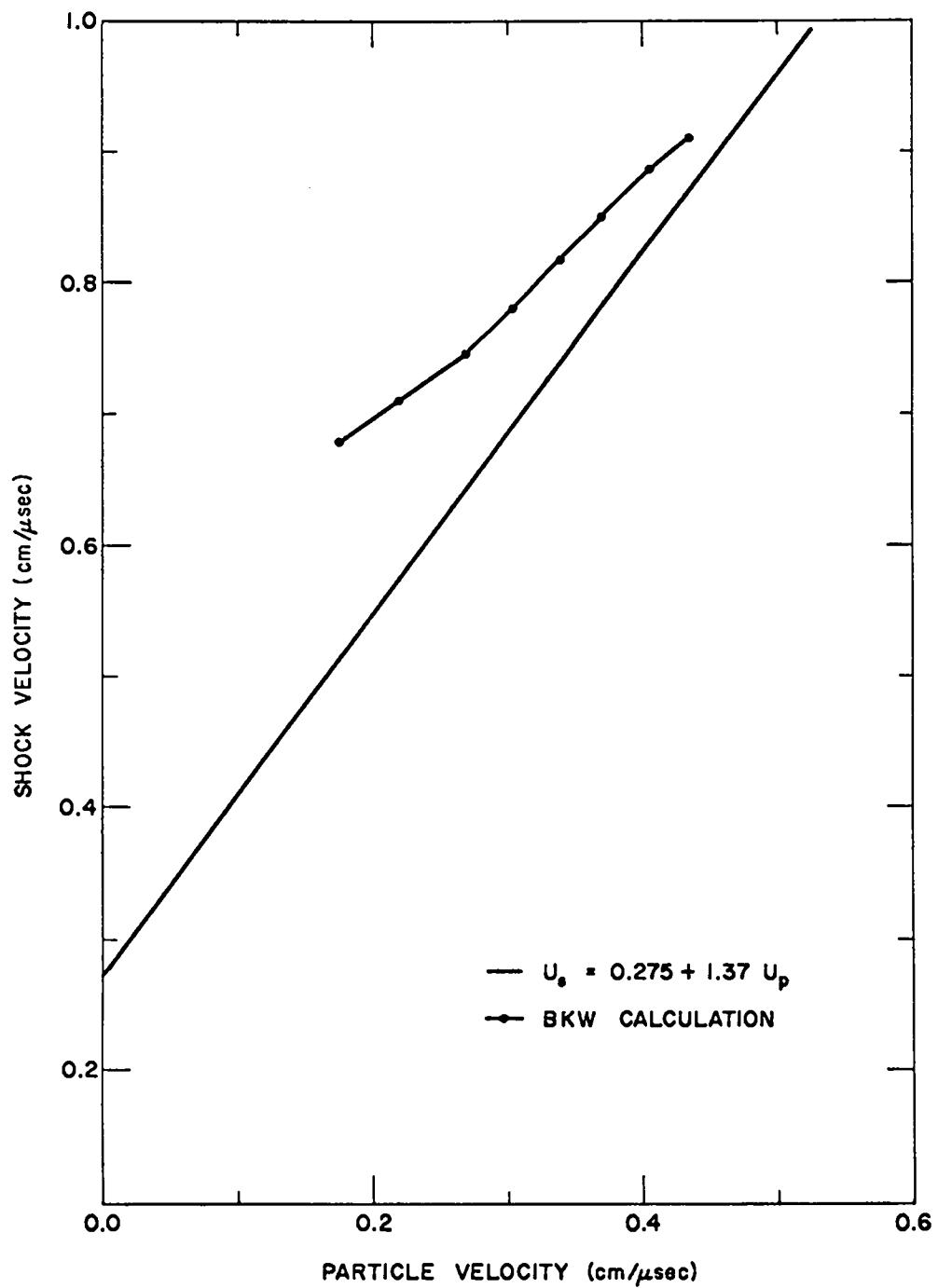
Fig. 4. The experimental and calculated Hugoniot curves for 1.265-g/cc polyurethane.
