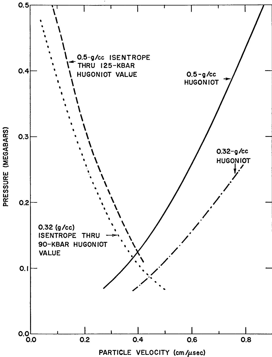
Fig. 3. The calculated BKW Hugoniots and isentropes for 0.5- and 0.32-g/cc polyurethane.
