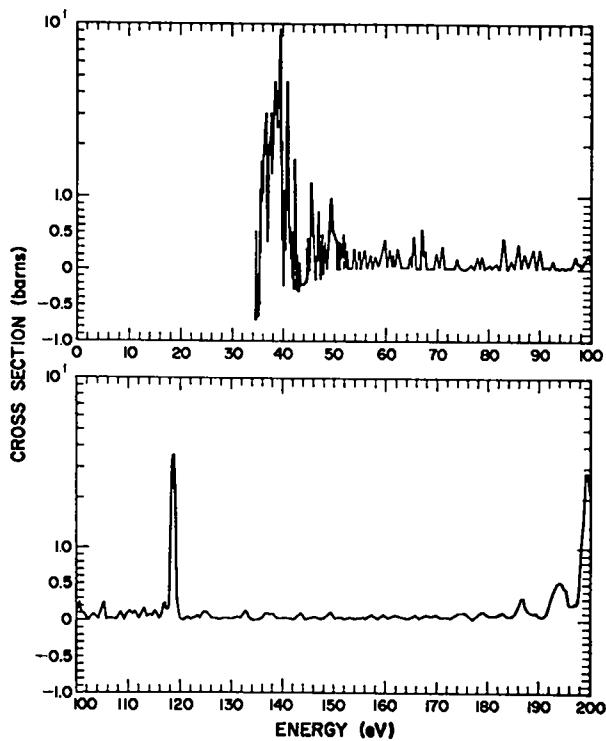
Fig. 1. The  $^{237}\text{Np}$  fission cross section 30 to 200 eV as measured in the Pommard experiment of March 1968. The time channel width  $\Delta t = 1.0 \mu\text{sec}$  or one-tenth of the Doppler width, whichever is larger.
