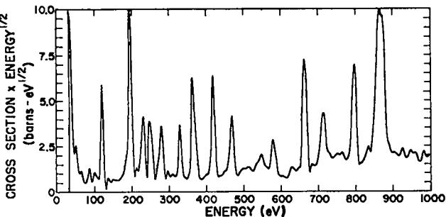
Fig. 4. The  $^{237}\text{Np}$  fission cross section times the square root of the neutron energy from 30 to 1000 eV (averaged over 7-eV intervals). The figure emphasizes the groupings of resonances.
