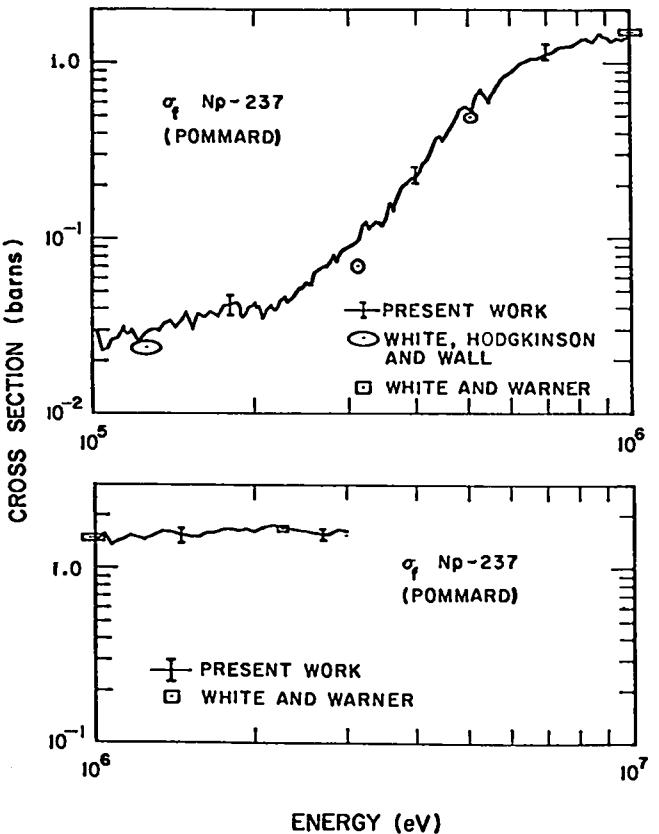
Fig. 3. The  $^{237}\text{Np}$  fission cross section 100 keV to 3 MeV.  $\Delta t = 0.2 \mu\text{sec}$ . The data of White and Warner,<sup>12</sup> and of White, Hodgkinson, and Wall<sup>13</sup> are included for comparison. The dimensions of the symbols represent the uncertainties in cross section and energy.
