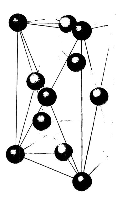
Fig. 1. The Unit Cell of Gamma Plutonium.
