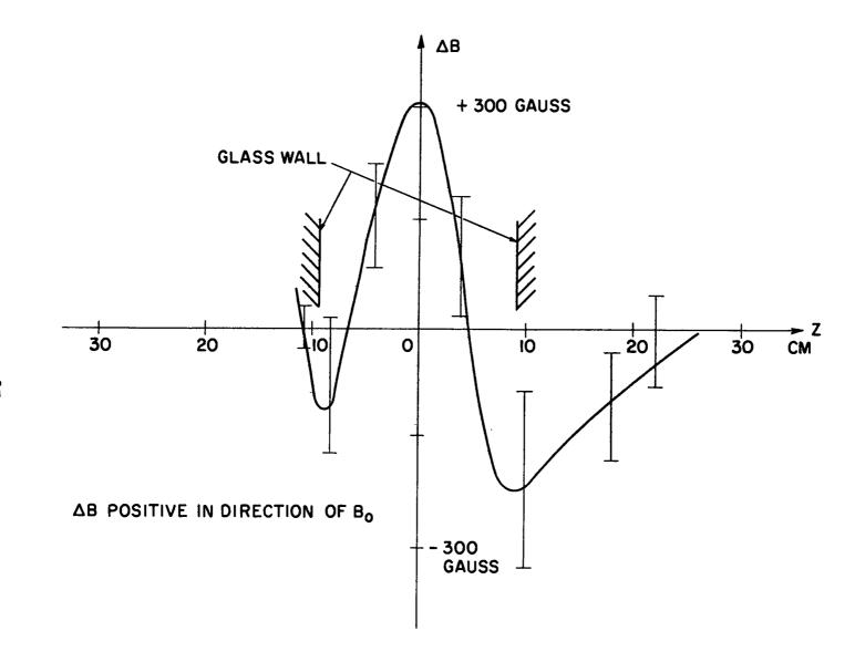
Fig. 2.  $\triangle B_z$  Distribution Indicated by Magnetic Probes
