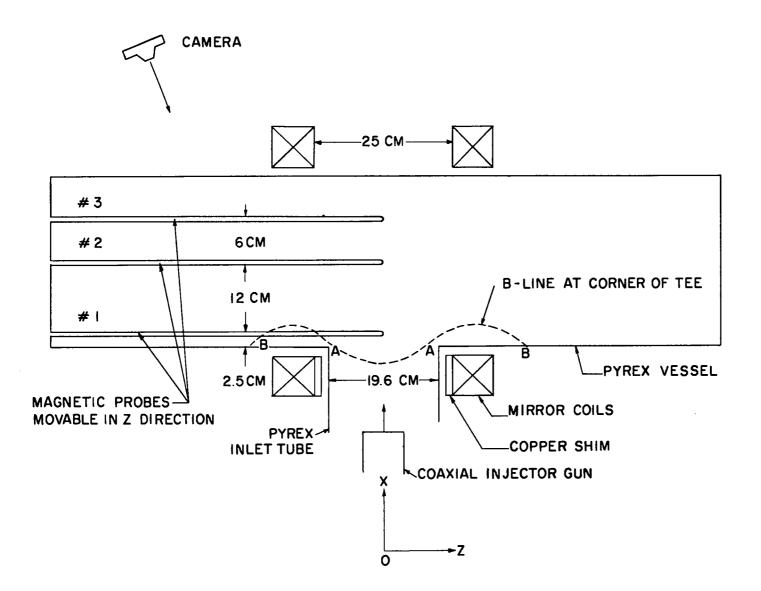
Fig. 1. Transverse Magnetic Field Injection
