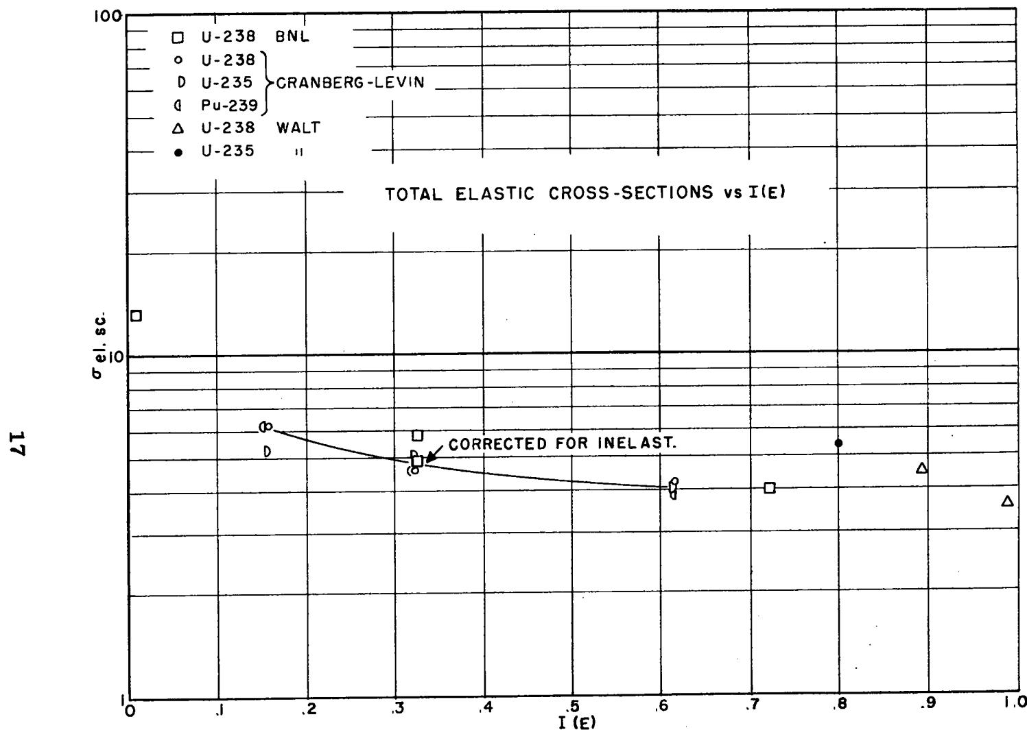
Fig. 6 Energy dependence of elastic scattering cross sections over the range of the fission neutron spectrum.
