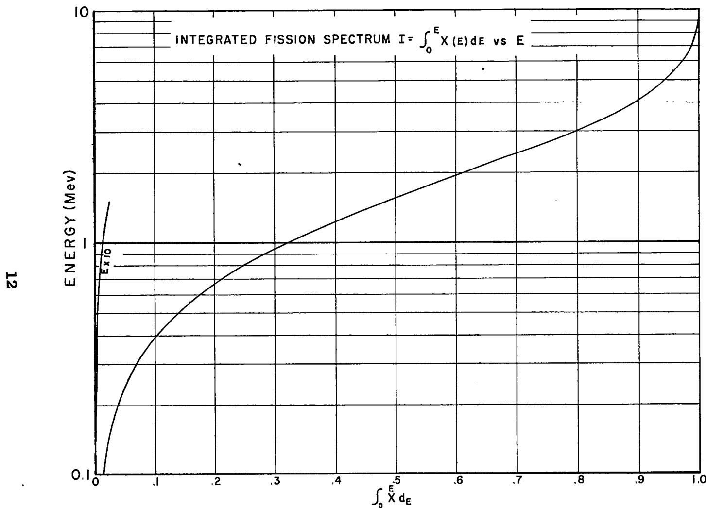
Fig. 1 Energy versus fraction of fission neutron spectrum below this energy.
