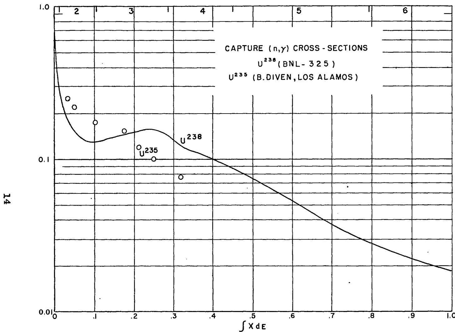
Fig. 3 Energy dependence of U-235 and U-238 capture cross sections over the range of the fission neutron spectrum.
