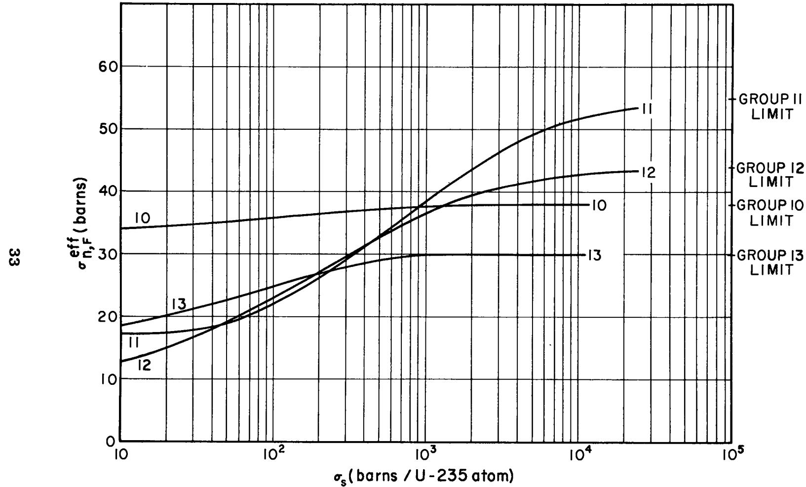
Fig. 11 Shielded fission cross sections for  $U^{235}$ .
