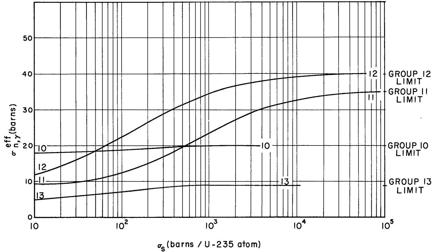
Fig. 10 Shielded capture cross sections for  $^{235}\text{U}$ .
