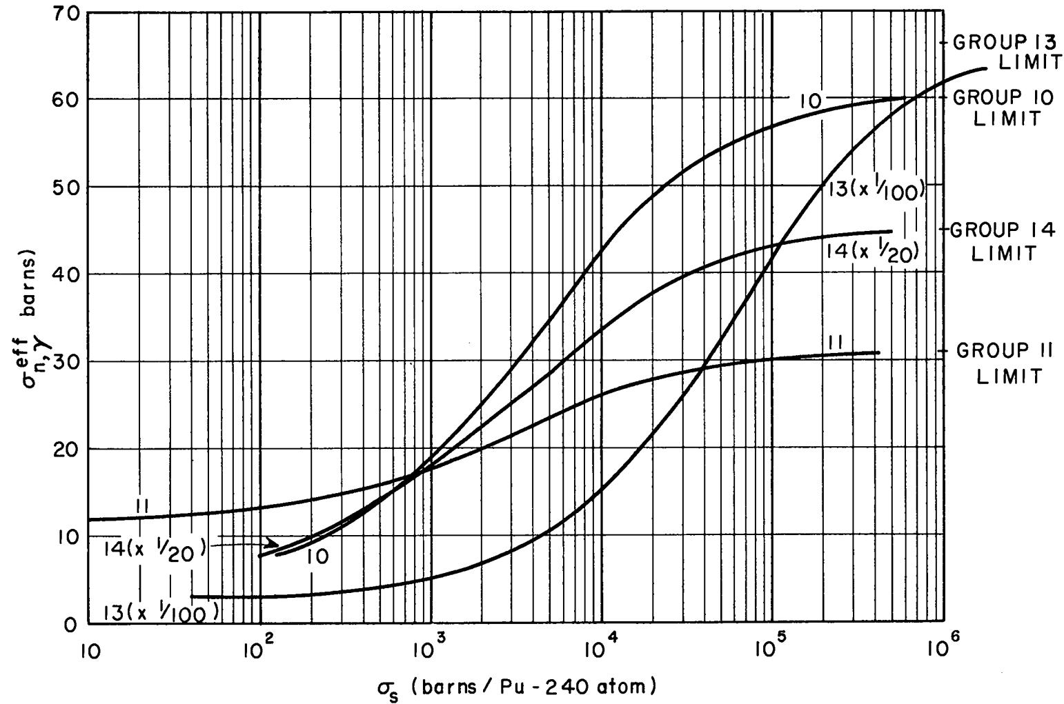
Fig. 9 Shielded capture cross sections for  $\text{Pu}^{240}$ .
