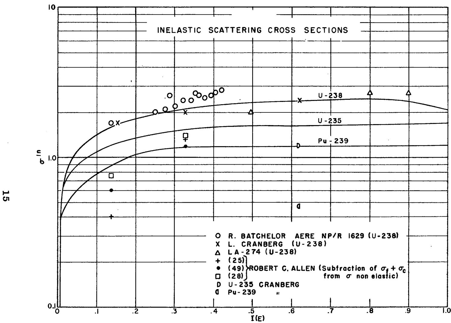
Fig. 4 Energy dependence of inelastic scattering cross sections over the range of the fission neutron spectrum.
