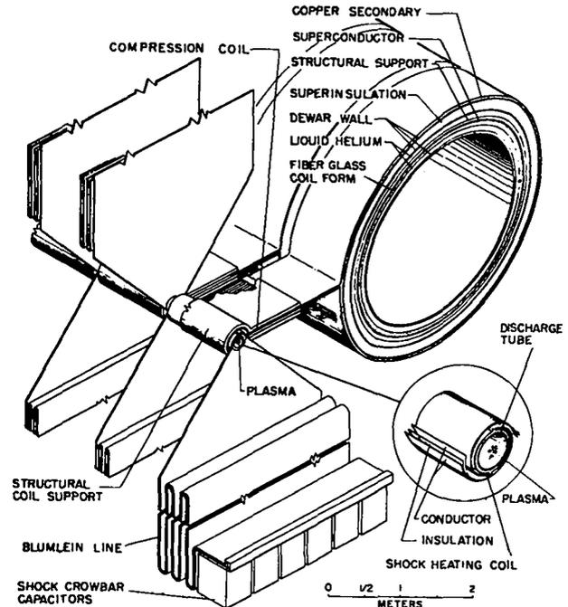
Fig. 12. Conceptual view of a portion of a separated-shock  $\Theta$  pinch.
