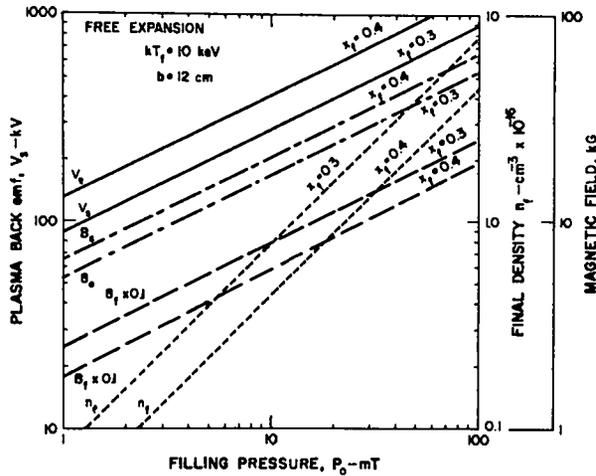
Fig. 4. Plasma heating parameters versus filling pressure for various compression ratios  $x_p$ . Free expansion of the ions after the initial implosion is assumed.
