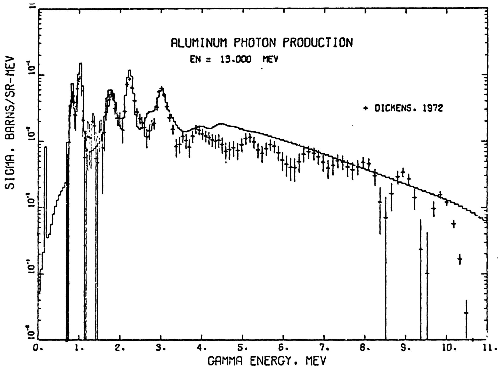
Fig. 3. Secondary gamma-ray spectrum at  $\theta = 125^\circ$  from the  $^{27}\text{Al}(n, \gamma)$  reaction with neutrons of energy 12-14 MeV. The curve is the ENDF/B(3) evaluation,<sup>4</sup> and the crosses represent the experimental data of Dickens et al.<sup>3</sup>
