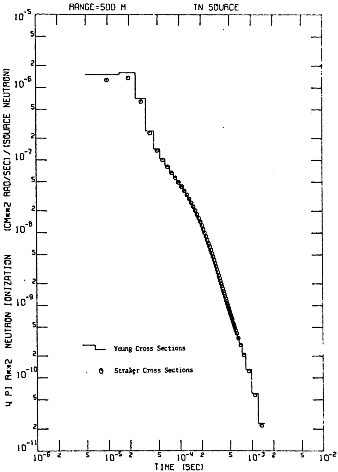
Fig. 6. Time-dependent neutron ionization in silicon at a range of 500m from a thermonuclear source as calculated by Engle and Mynatt.<sup>20</sup> <sup>14</sup>N and <sup>16</sup>O evaluations by Young and Foster<sup>2,24</sup> and by Straker and Gritzner<sup>21</sup> were used in the calculations.
