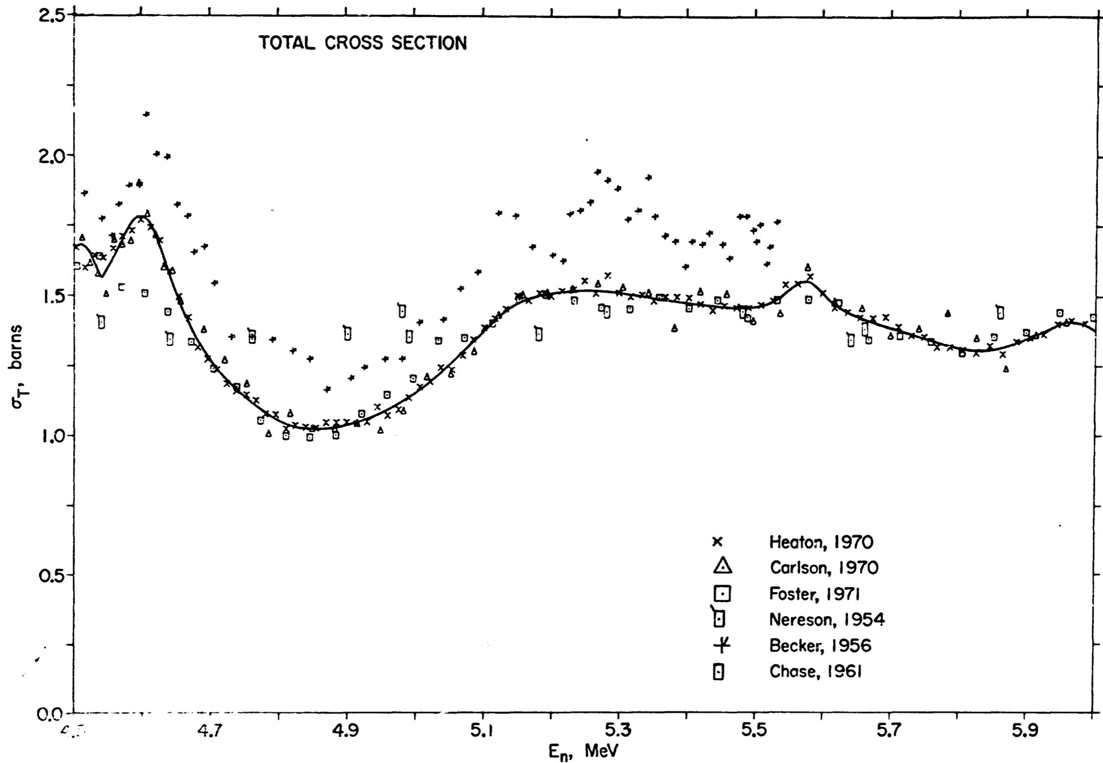
Fig. 5. Measured and evaluated  $^{14}\text{N}$  total cross section from 4.5 to 6.0 MeV. The experimental data of Heaton,<sup>14</sup> Carlson,<sup>15</sup> Foster,<sup>16</sup> Nereson,<sup>17</sup> Becker,<sup>18</sup> and Chase<sup>19</sup> are compared to the ENDF/B(3) evaluation.<sup>2</sup>
