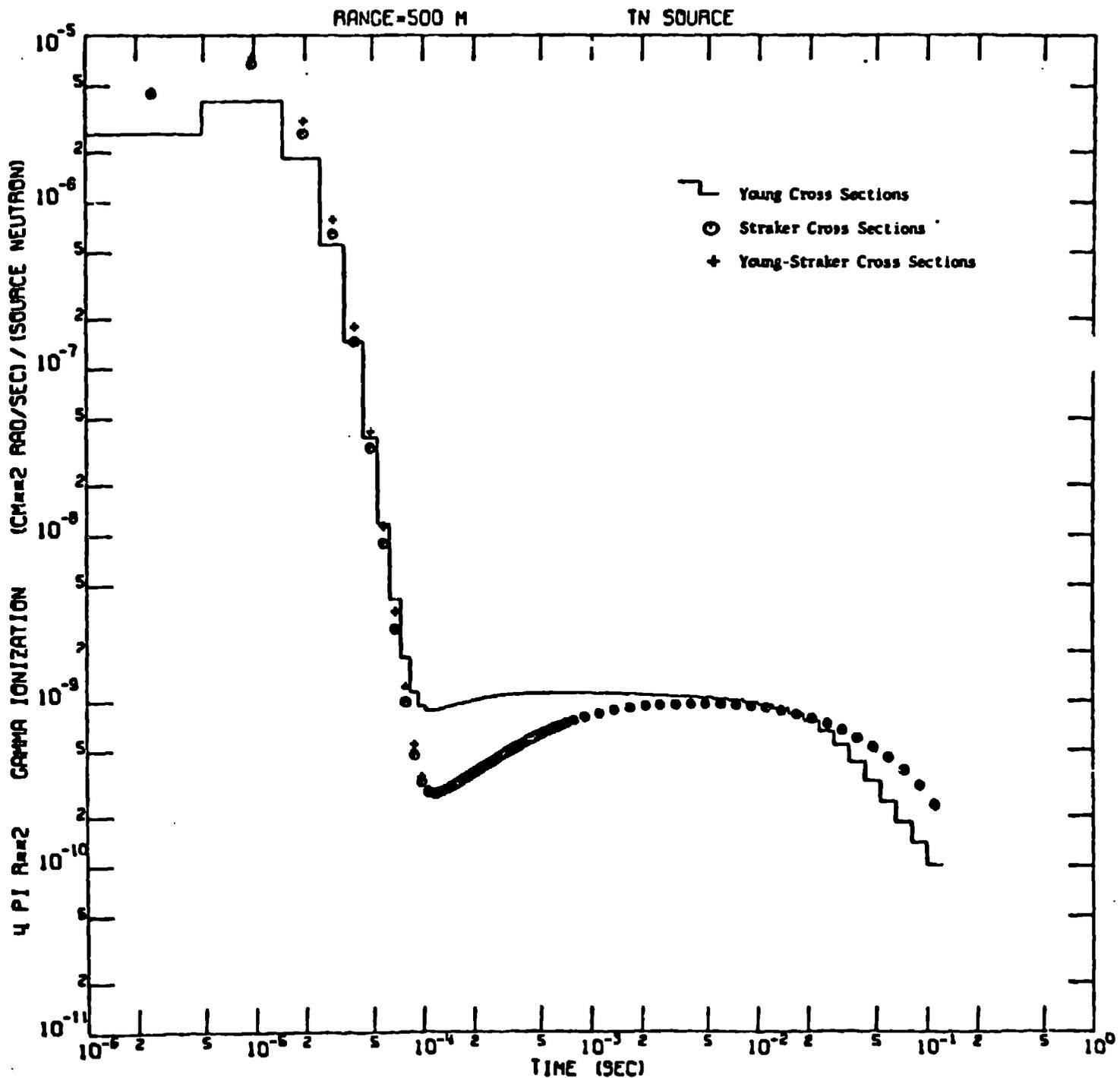
Fig. 7. Time-dependent gamma-ray kerma in silicon at a range of 500m from a thermonuclear source as calculated by Engle and Mynatt.<sup>20</sup> The calculations were performed using data evaluations by Young and Foster,<sup>2,24</sup> Straker and Gritzner,<sup>21</sup> and a hybrid set consisting of the neutron data from Young and Foster and the gamma-ray production data from Straker and Gritzner.
