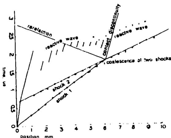
FIGURE 7. x-t DIAGRAM FOR PBX 9404 EXPT.
