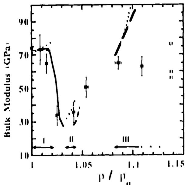
Figure 1. Bulk modulus to shocked Carrara marble (squares) versus normalized density compared with hydrostatic data (see text)
