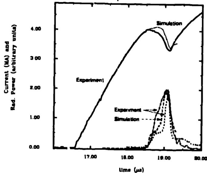
Fig. 6. Experimental current (solid) and two XRD radiation measurements (dot-dash and short-dash, representing two energy filterings) compared with a 2-D simulation current (dot) and radiation power (long-dash) for the the second 13.0 mg implosion experiment. Current is shown in MA, and the XRD signals and radiation power have been scaled to a peak value of 2.0 in arbitrary units.
