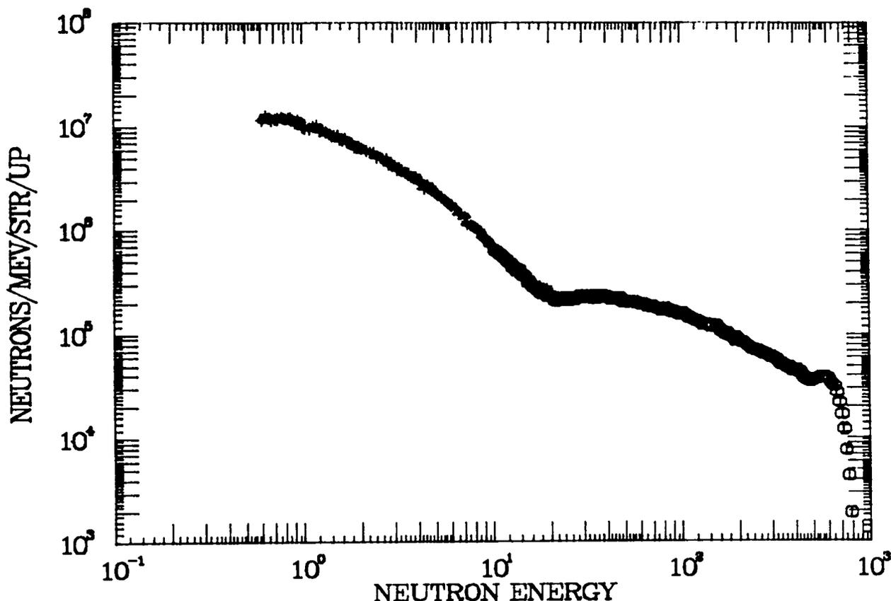
Fig. 5. The neutron flux obtained at the 15° flight paths. These results are based on the known  $^{235}\text{U}$  cross section below 20 MeV. The circles are the neutron flux obtained from the plastic scintillator which is normalized to the absolute flux in the overlap energy range from 10 to 20 MeV.
