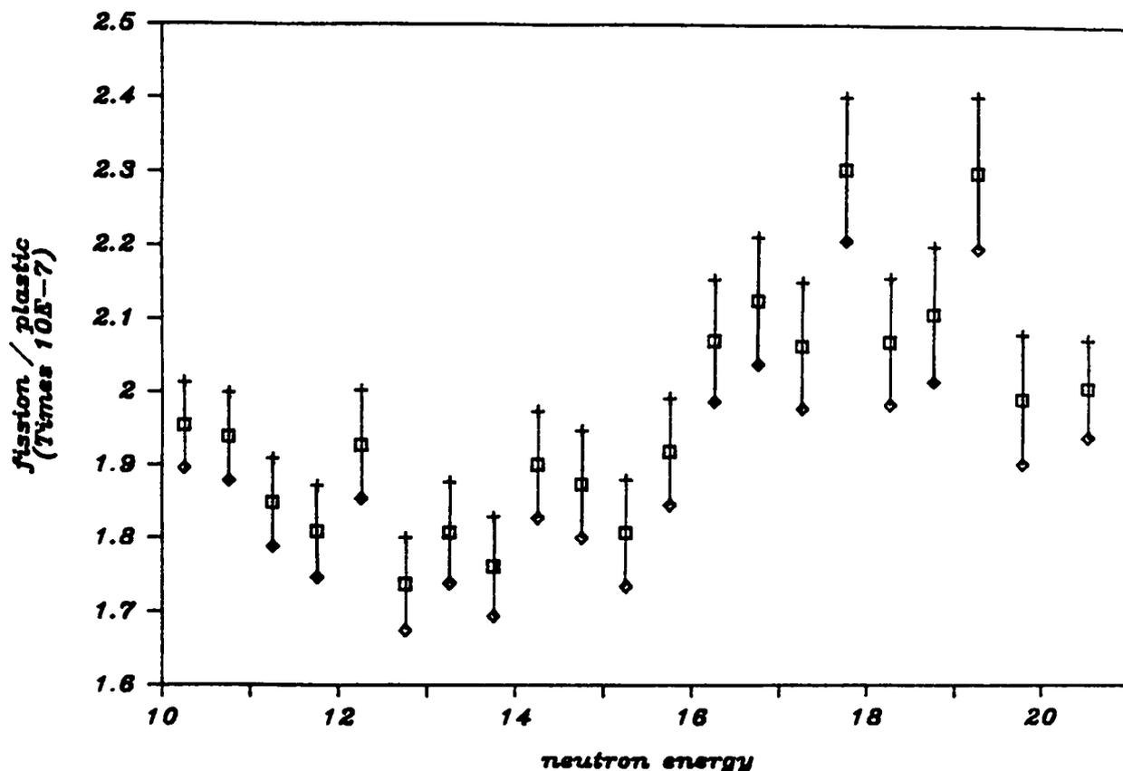
Fig. 4. The ratio of the absolute neutron flux measured using the fission chamber to the relative flux measured using the plastic scintillator in the overlap energy region from 10 to 20 MeV.
