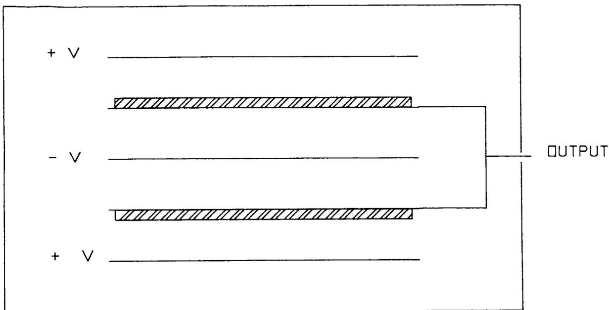
Fig. 1. Diagram of the fission chamber used in measuring the neutron flux at Target-4 and the  $^{235}\text{U}$  fission cross section. The uranium deposits are shown in the cross hatched region.
