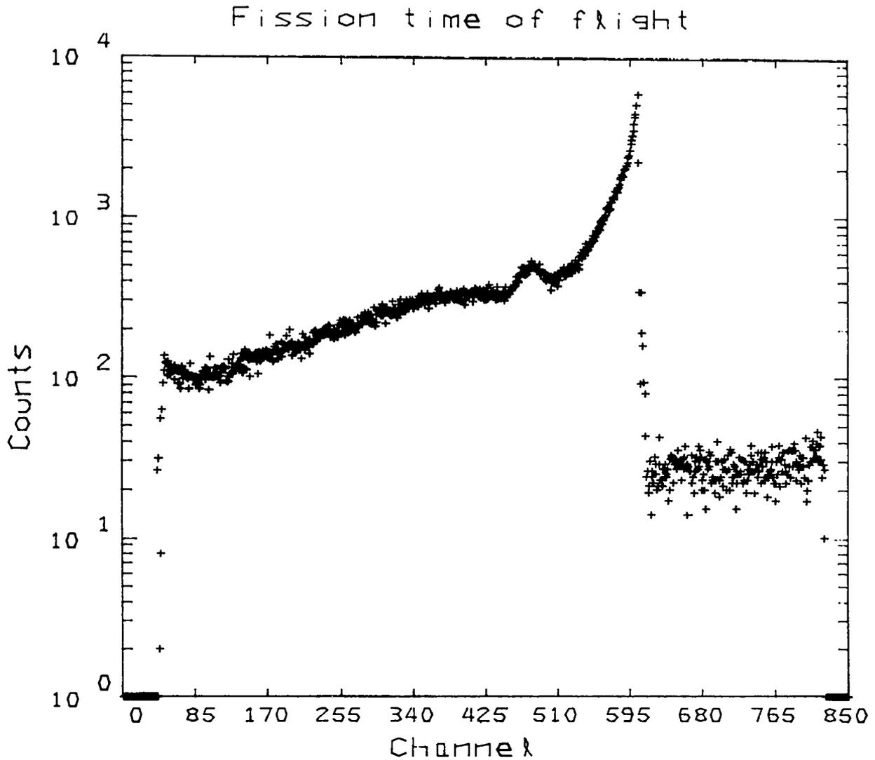
Fig. 2. Typical time-of-flight spectrum for the fission chamber.
