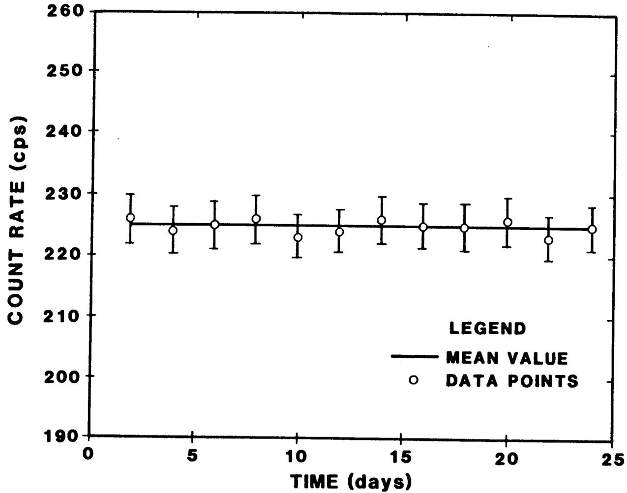
Figure 2.7 Long Term Stability of the NaI (Tl) Spectrometer
