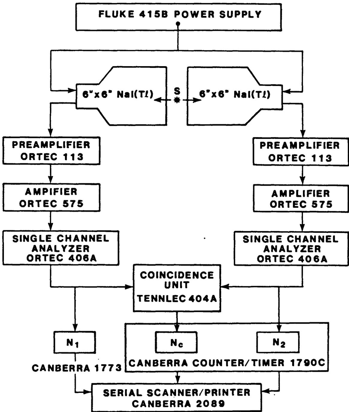
Figure 2.4 Schematic Diagram of the NaI (Tl) Spectrometer
