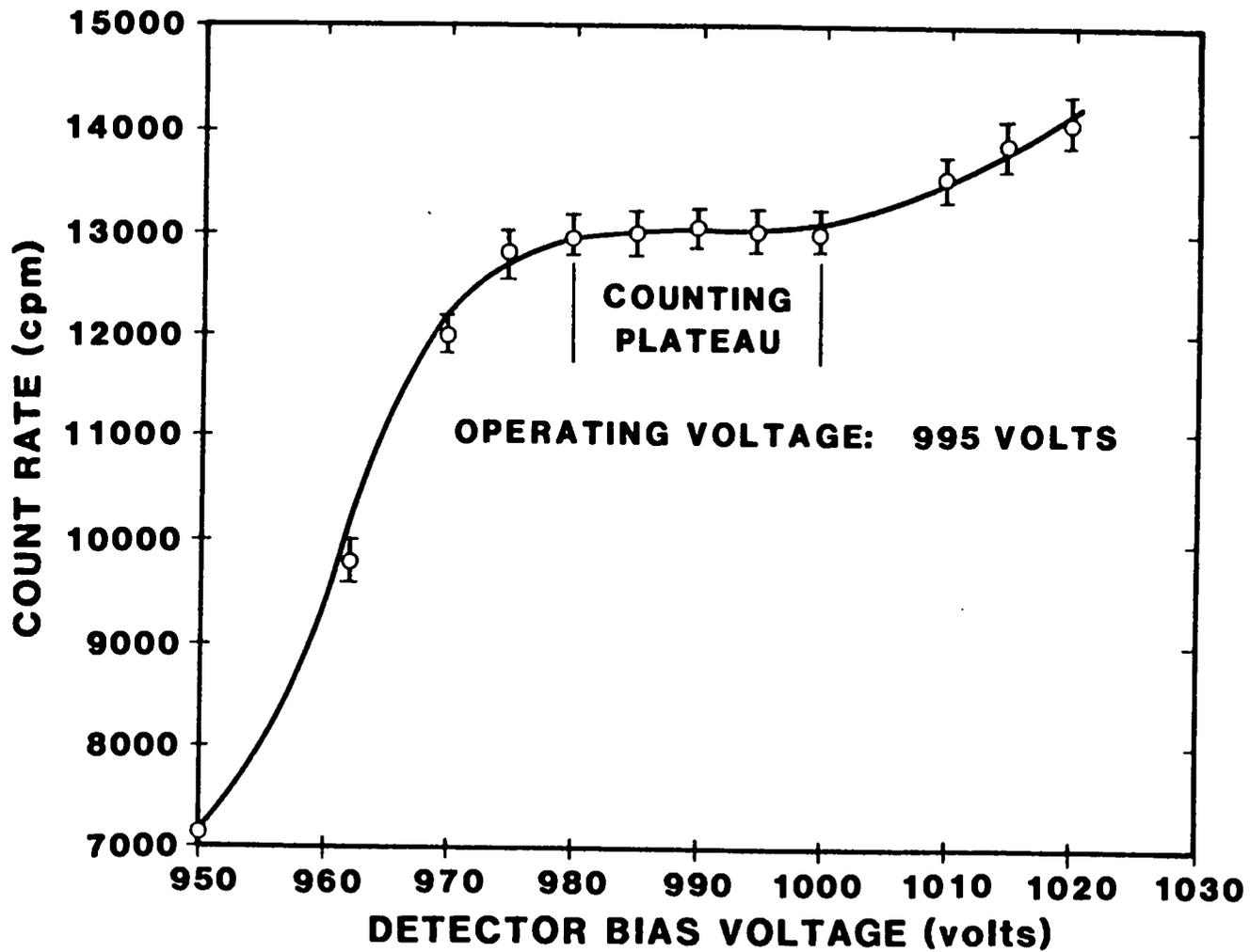
Figure 2.5 Counting Plateau Determination NaI (Tl) Spectrometer
