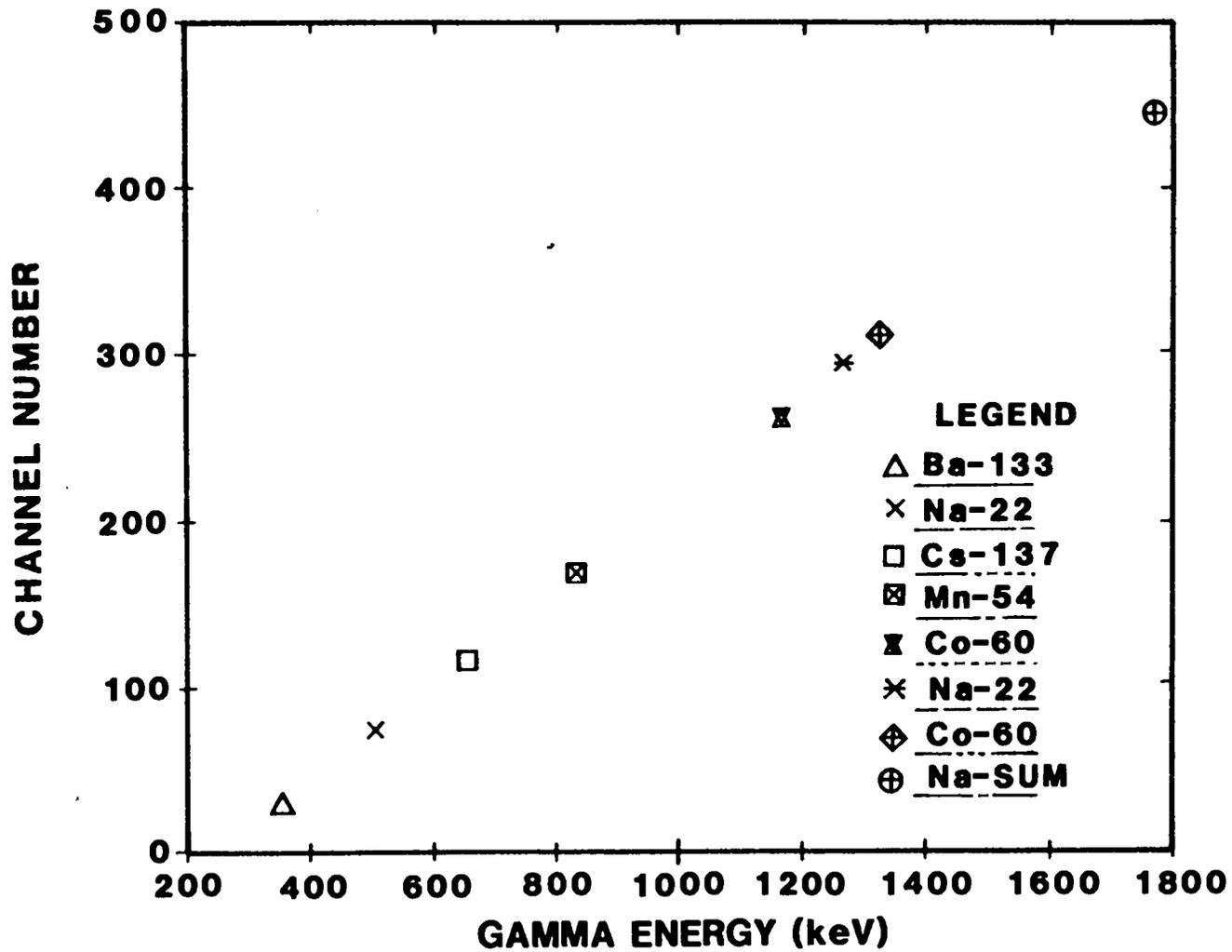
Figure 2.6 Energy Calibration of the Multichannel Analyzer Canberra Series 30
