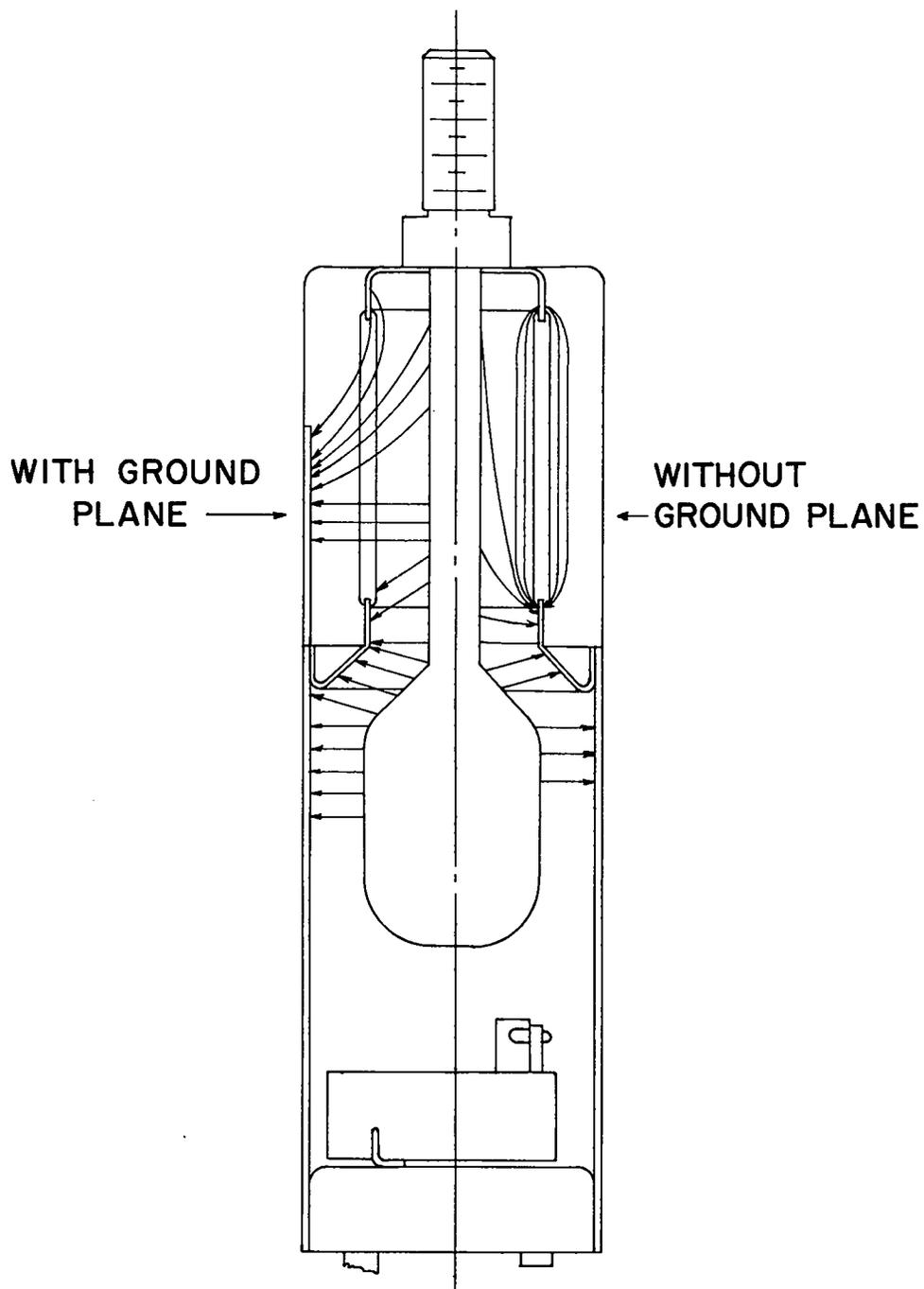
Fig. 7. Flux plots with and without ground plane
