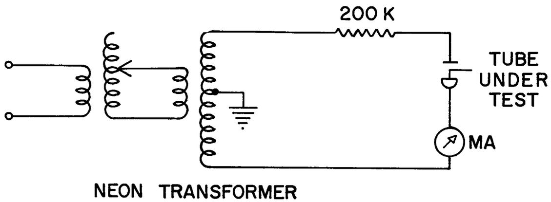
Fig. 1. AC Hy-Pot circuit
