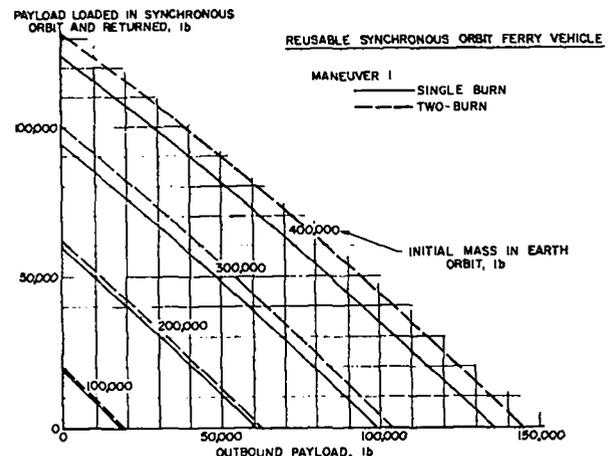
Fig. 13. Effect of two-burns for Maneuver 1.
