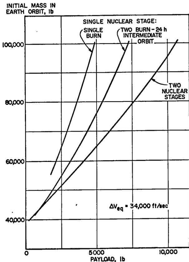
Fig. 7. Vehicle requirements for a 34 000 ft/sec mission.
