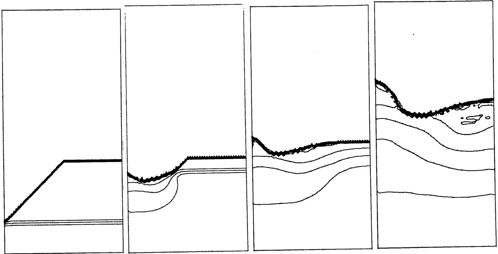
Fig. 8. The isopycnics for the computed interaction of a shock in water with a 1-cm-deep V notch at 1.0, 2.5, 3.5, and 5.0  $\mu\text{sec}$ . A constant-pressure, 121-kbar piston is assumed, and the apex of the notch is 0.5 cm above it.
