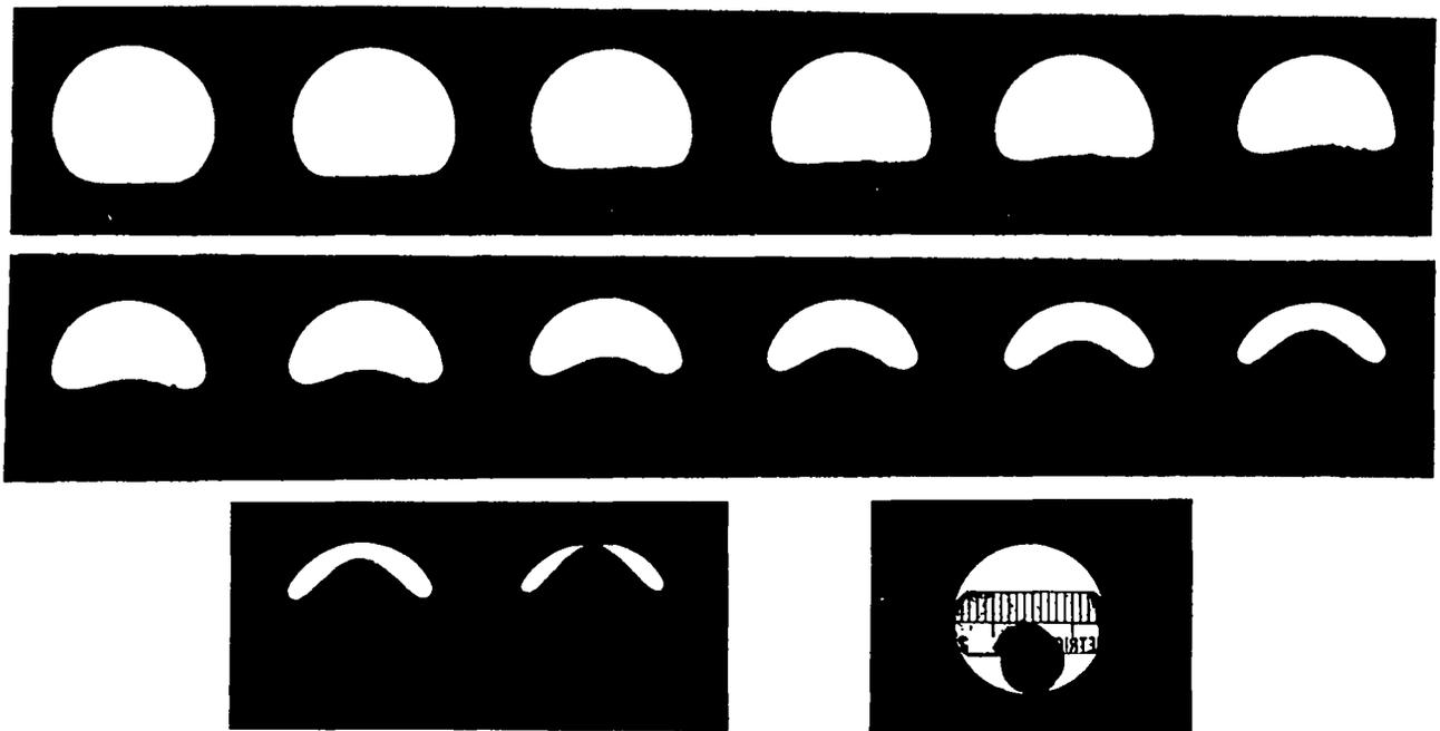
Fig. 14. Framing-camera photographs of the closure of a 1-cm-radius cylindrical void in polyethylene in the same geometry as that in Fig. 13. Time between frames is 0.21  $\mu$ sec, and exposure time is 0.09  $\mu$ sec. The last frame is a still photograph.
