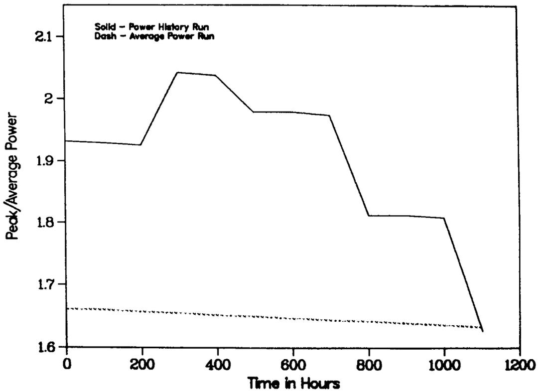
Fig. 34. Effect on peak/average power ratio in Driver-2.
