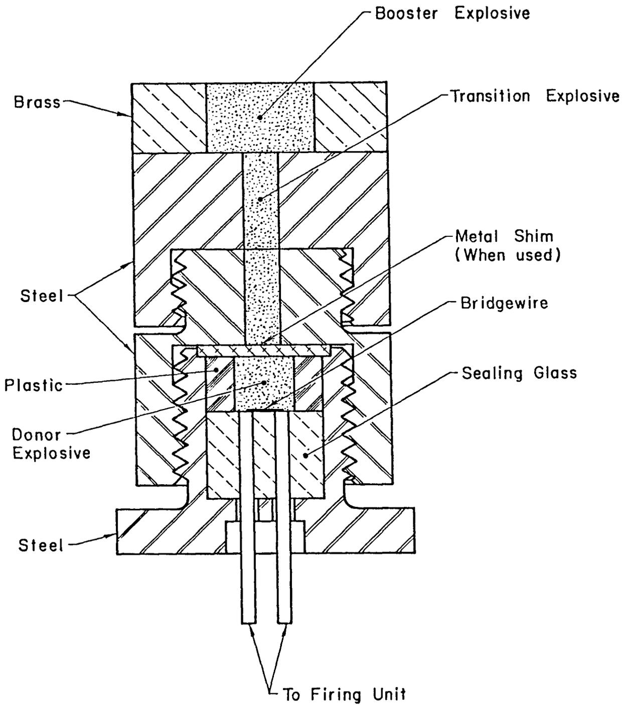
Fig. 1. DDT Assembly (ER-322 type).
