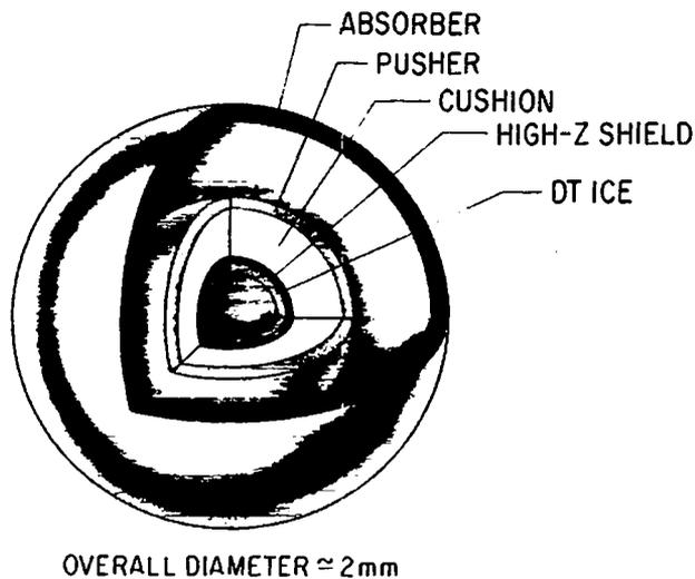
Fig. 2. Example of a Dagwood target with six shells.
