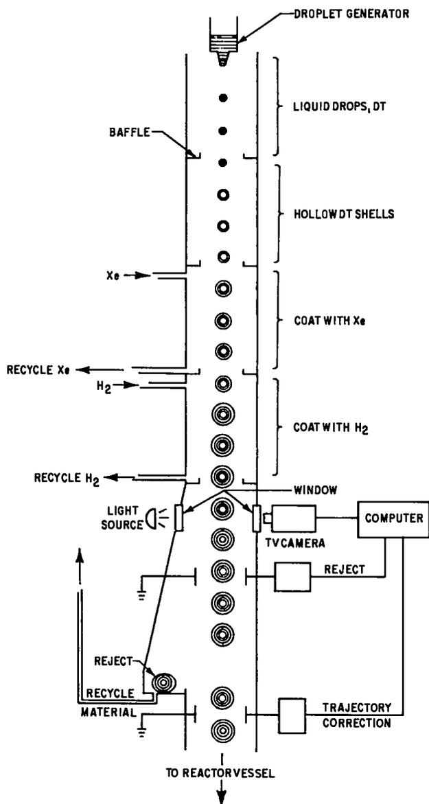
Fig. 5. Drop tower for making special cryogenic targets.
