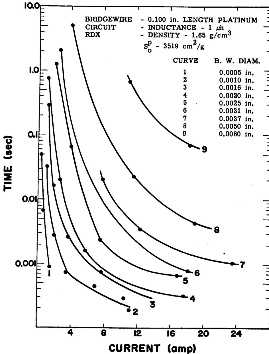
Fig. 3. Current versus current duration for hot-wire ignition of RDX in a Type 2 pressure cartridge.
