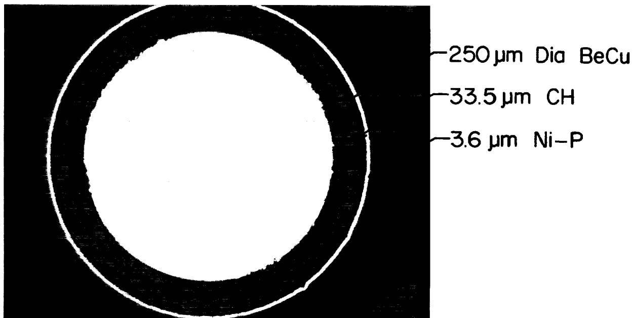
Fig. VII-26. Target for hot-electron measurements.
