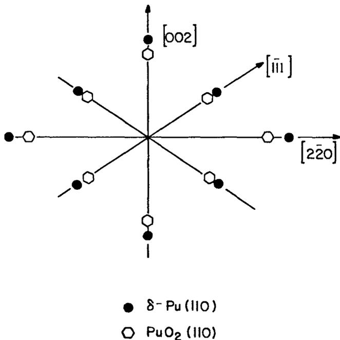
Fig. 6. Schematic (110) SAD showing indexing of diffraction spots for Pu-1.5 wt% Ga and the epitaxial  $\text{PuO}_2$ .
