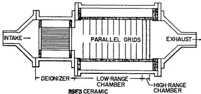
Fig. 1. Schematic of a wide-range tritium monitor.
