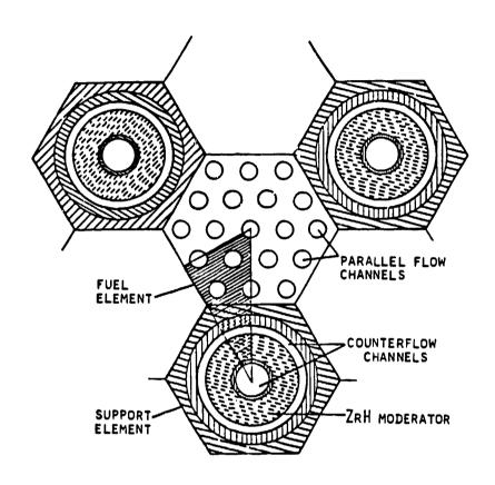
Fig. 8. Gas-cooled space nuclear power system fuel-support element cluster configuration (see Fig. 7) analyzed with the OPTION thermal-fluid code. Analysis based on triangular region of symmetry that is shaded, see Fig. 9.
