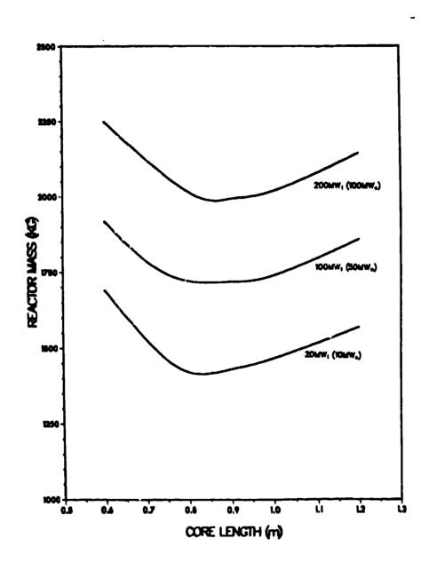
Fig. 17. Core length versus reactor mass for several power levels based on the thermal-fluid and neutronic analytical results given in Fig. 16.
