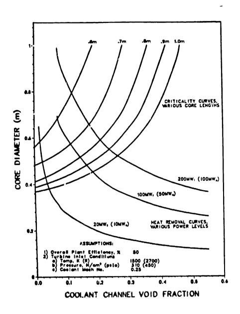
Fig. 16. Thermal-fluid and neutronic analysis results. A mass analysis at the intersections of these results is shown in Fig. 17.
