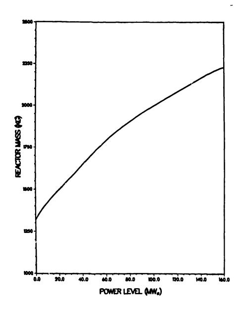
Fig. 18. Power level versus reactor mass corresponding to the minimum core diameters for the curves of Fig. 17.
