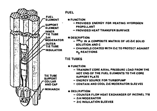
Fig. 7. Rover program Small-Engine reactor fuel model. See figs. 2, 5 and 6.
