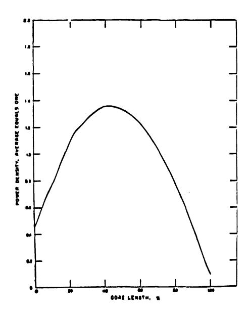
Fig. 13. Axial power profile used for OPTION thermal-fluid analysis.
