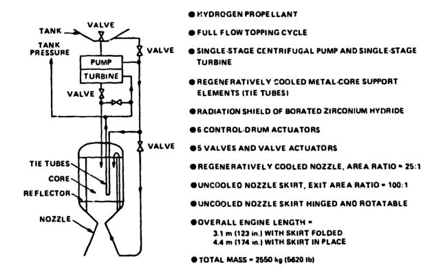
Fig. 5. Rover Small-Engine flow diagram and general description. Note that the tie-tube coolant is used to operate the turbine that pumps the propellant.
