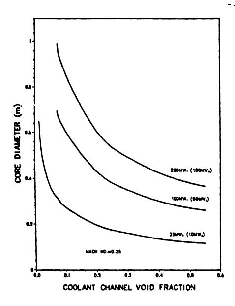
Fig. 12. Reactor core diemeter (m) versus coolant channel void fraction for several power levels. MWt is thermal power level and MWe is electrical power level. (conversion efficiency is 0.50). The calculations are for an inlet temperature of 370 K (666 R) and exit conditions of 1500 K (2700 R), 3.10 MPa (450 psia) and Mach number of 0.25.
