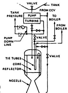
Fig. 4. Dual-mode nuclear rocket flow diagram showing use of tie-tube support thermal energy for low-power electrical mode.
