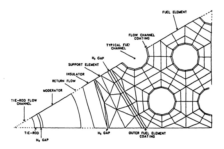
Fig. 9. Finite-element mesh for the OPTION-code determination of transverse conduction and temperature distribution for the cluster configuration shown in Fig. 7. Note that the model includes representation of the coatings, possible gaps, and a complicated geometry. Geometric specification is exhitrary, i.e., the coolant diemeters, coatings and gap thickness, hole spacing, etc. are input.
