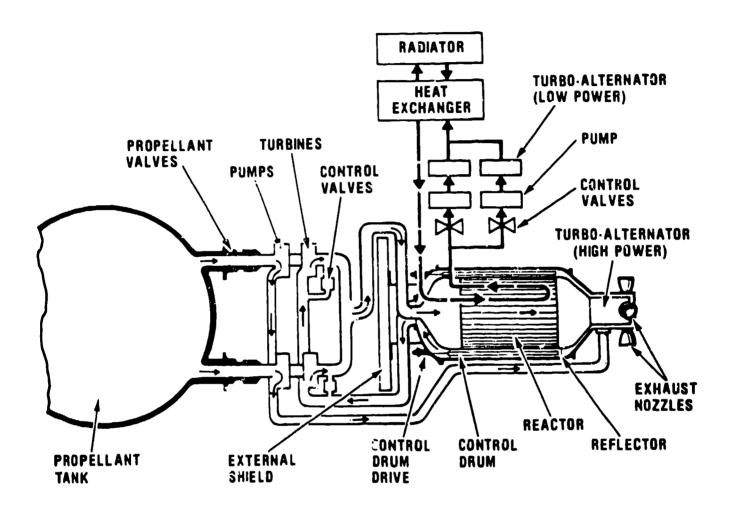
Fig. 3. Dual-mode Rover power plant flow diagram. Note the recirculation loop through the tie -tube supports provides steady-state low power for station keeping.
