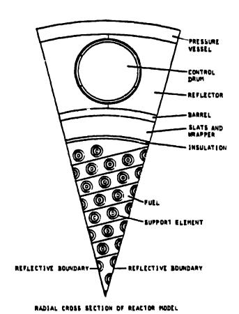
Fig. 15. Monte Carlo neutron and photon transport code radial cross section of reactor.
