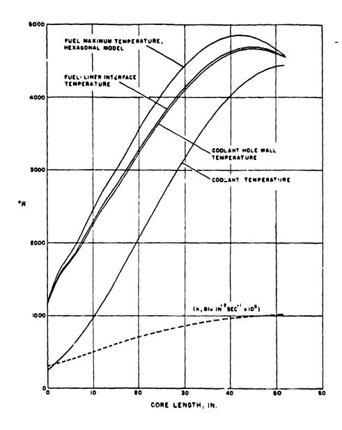
Fig. 14. Typical OPTION thermal-fluid code temperature and heat-transfer coefficient versus core length profiles.
