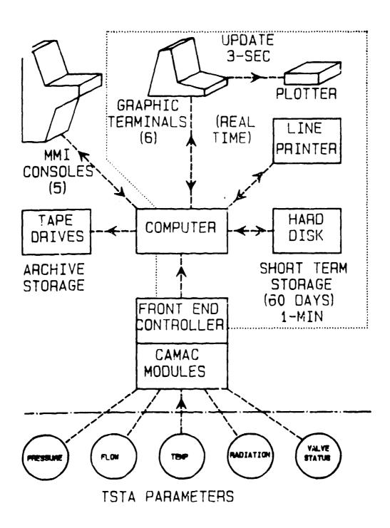
Fig. 5. Using the computer TREND program to correlate a tritium leak with a specific pressure sensor.
