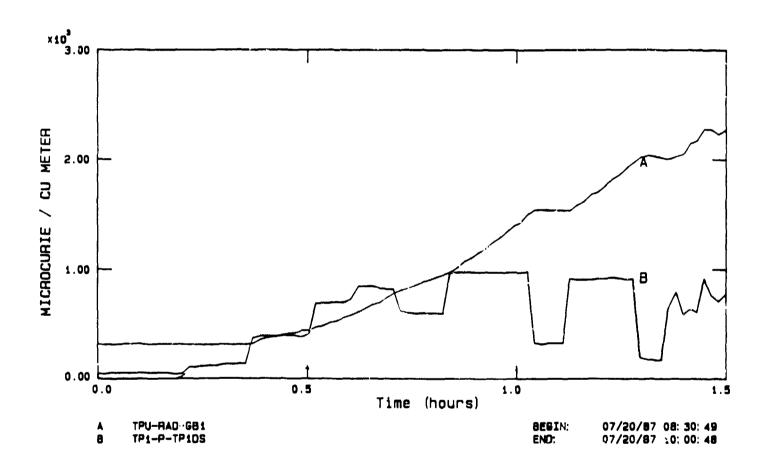
Fig. 6. Leak testing in a glovebox, using an external tritium detector and pump.
