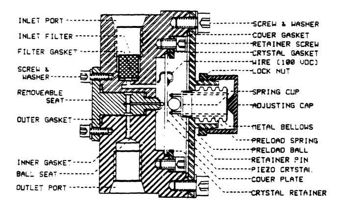
Fig. 1. The TFTR tritium-hardened piezoelectric valve.
